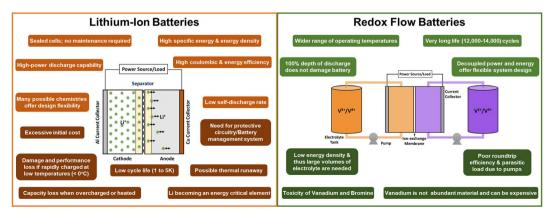
Fig. 4 Comparison of lithium-ion and redox flow batteries.
