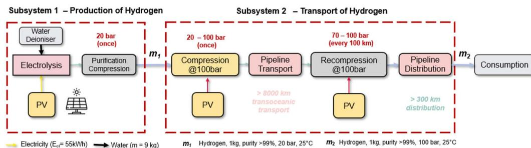
Fig. 3 System boundaries of hydrogen transport. Left – subsystem 1: production of hydrogen; right – subsystem 2: transport of hydrogen.
