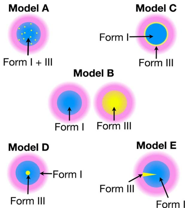
Fig. 2 Models A–E show different possible distributions of the two *m*-ABA polymorphs, Form I and Form III. The solution (pink) containing the polarizing agent is located on the surface of the particles. Numerical simulations of  $^1\text{H}$  spin diffusion suggested that model B best reproduced the DNP saturation recovery experiments. Reproduced with permission from ref. 15.
