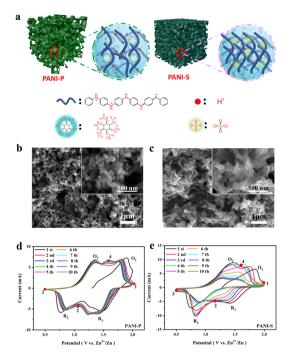
Fig. 1 (a) Microscopic schematic diagram of different PANI doped acids; scanning electron microscopy images of different PANI doped acids: (b) doped phytic acid; (c) doped sulfuric acid; cyclic voltammetry curve (CV curve) sweep rate of 10 mV s<sup>-1</sup> for different PANI doped acids: (d) PANI doped phytic acid electrode in 1 M zinc sulfate electrolyte with addition of zinc phytate (1%); (e) PANI doped sulfate electrode in 1 M zinc sulfate electrode in 1 M zinc sulfate electrodyte.
