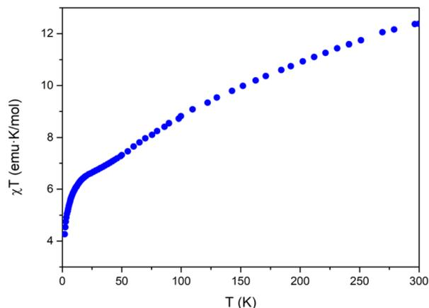
Fig. 2 Thermal behavior of  $\chi_{\text{T}}$  for  $\text{Na}[\text{Co}_2\text{Fe}_2\text{-WS}]$  at 0.1 T field in the range 2–300 K.
