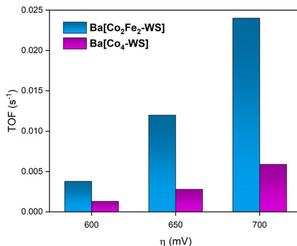
Fig. 9 Comparison of the calculated TOFs of **Ba[Co<sub>2</sub>Fe<sub>2</sub>-WS]** and **Ba[Co<sub>4</sub>-WS]** at different overpotentials during RDE-LSV measurements. The experiments were conducted using 30 wt% Ba[POM]/CP electrodes at pH = 7.2 using 50 mM KP<sub>9</sub> buffer and KNO<sub>3</sub> (1 M) as aqueous electrolyte. The scan rate was 1 mV s<sup>-1</sup> and the rotational speed was 1600 rpm.
