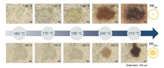
Fig. 6 In situ optical microscopy of polypropylene (PP) cracking using FCC catalyst. Individual polymer grains were placed on a bed of FCC catalyst and heated at 10 °C min<sup>-1</sup> under  $N_2$  flow in a Linkam stage. Images were acquired every minute. See ESI† for videos of the full reaction. Top:  $PP_{23k}$ . Bottom:  $PP_{307k}$ .
