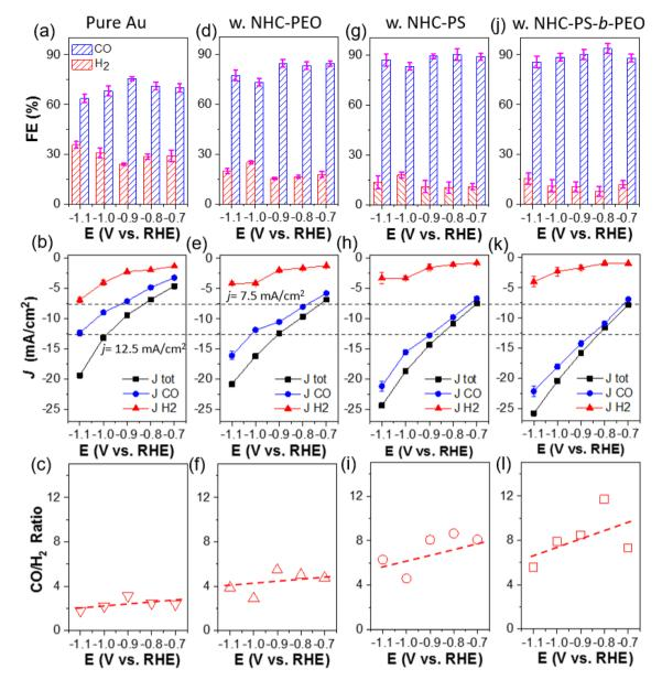
Fig. 2 Electrocatalytic performance of  $CO_2$  reduction on different catalysts: FE, (partial) current density and product ratio (ordered vertically) using pure Au (a)–(c), Au–P1 (d)–(f), Au–P2 (g)–(i) and Au–P3 (j)–(l). All tests were carried out in  $CO_2$  saturated 0.1 M KHCO<sub>3</sub>.
