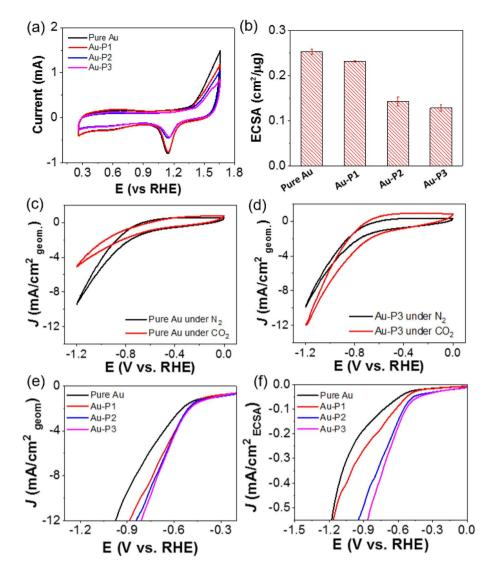
Fig. 1 (a) CVs of Au/C with different polymer ligands measured in  $N_2$ -saturated 0.5 M  $H_2SO_4$  with a scan rate of 100 mV  $s^{-1}$ . (b) ECSAs of AuNPs modified with various ligands. (c) and (d) CV curves of AuNPs (c) and Au-P3 (d) under N2 (black) and CO2 (red). (e) and (f) LSV curves measured in CO<sub>2</sub>-saturated 0.1 M KHCO<sub>3</sub> at a scan rate of 10 mV s<sup>-1</sup> normalized to (e) geometric area of electrodes and (f) ECSA of AuNPs
