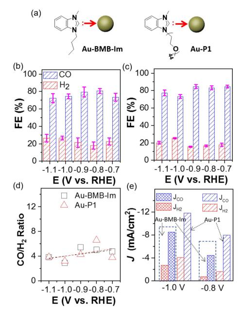
Fig. 3 (a) Scheme of BMB-Im and PEO-NHC modified AuNPs through Au-C binding. Catalytic selectivity to CO and H<sub>2</sub> using Au-BMB-Im (b) and Au-NHC-PEO (c). (d) Product ratio and (e) current density analysis of Au-BMB-Im and Au-NHC-PEO.
