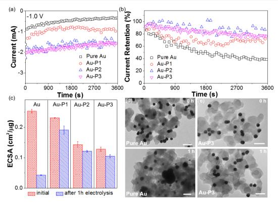
Fig. 7 Stability measurement using i-t curves (a), current retention (b) and ECSA (c). The experiments were carried out using constant-potential electrolysis at -1.0 V for 1 h. TEM images of pure Au (d) and Au-P3 (e) loaded on carbon before (top) and after (bottom) CO<sub>2</sub> electroreduction for 1 h. All scale bars are 40 nm.
