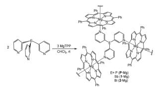
Scheme 2 Synthesis of the complexes  $\{[P(3-py)_3]_2 \cdot (MgTPP)_3\}_n \cdot (P \cdot Mg)$ ,  $\{[Sb(3-py)_3]_2 \cdot (MgTPP)_3\}_n (1 \cdot Mg) \text{ and } \{[Bi(3-py)_3]_2 \cdot (MgTPP)_3\}_n (2 \cdot Mg).$
