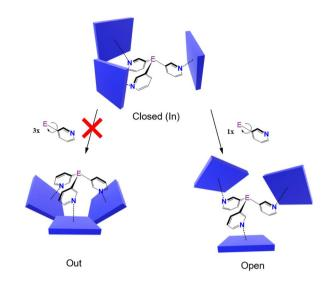
Fig. 3 Possible conformations of capsules of the type [(E(3-py) $_3$ )·(ZnTPP) $_3$ ].
