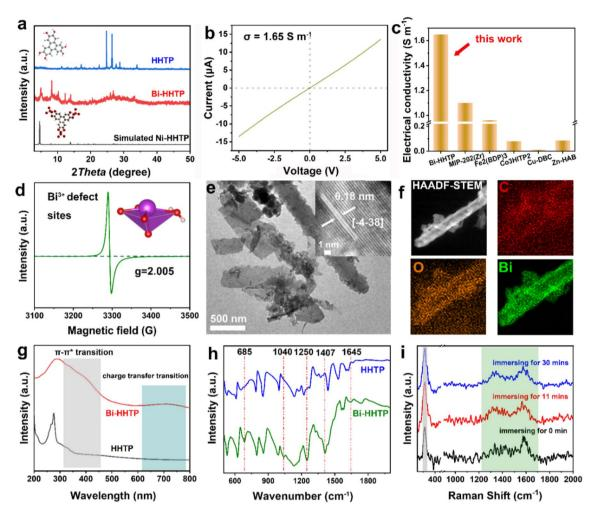
Fig. 2 (a) XRD patterns of Bi-HHTP and HHTP. (b) Current-voltage characteristic of Bi-HHTP using the two-contact probe method. (c) The compassion of conductivity of different MOFs. (d) EPR spectrum of Bi-HHTP. (e) TEM image, (f) HAADF-STEM image and the corresponding EDS elemental mappings of Bi-HHTP. (g) UV-vis spectra of Bi-HHTP and HHTP. (h) FTIR and (i) *in situ* Raman spectra of Bi-HHTP.
