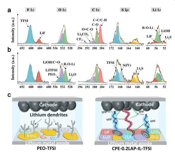
Fig. 5 High-resolution spectra of F 1s, O 1s, C 1s, S 2p, and Li 1s for Li electrodes dissembled from (a) Li||PEO-TFSI||Li and (b) Li||CPE-0.2LAP-IL-TFSI||Li cells after cycling at 0.1 mA cm<sup>-2</sup> for 50 h; (c) schematic illustration of lithium dendrites formation, chemical components on lithium metal anode and Li<sup>+</sup> transference pathway within ASSLMBs with PEO-TFSI or CPE-0.2LAP-IL-TFSI membranes.
