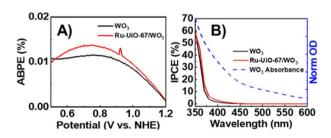
Fig. 3 (A) Photo-response efficiency of WO $_3$  (black) and Ru-UiO-67/WO $_3$  (red) as a function of potential (ABPE). (B) Wavelength (IPCE) of WO $_3$  (black), Ru-UiO-67/WO $_3$  (red) measured under monochromatic light at 500 mV applied potential, overlaid WO $_3$  absorption spectrum (blue dashed line).
