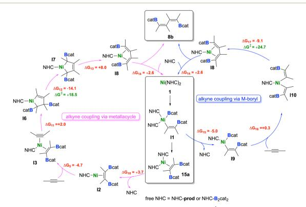
Scheme 8 Proposed catalytic cycles for the formation of 8b. Reaction free energies (kcal mol<sup>-1</sup>) calculated at the DFT level are shown in red, while energy barriers are shown in green (see ESI† for more details).
