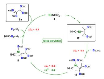
Scheme 7 Proposed catalytic cycle for the formation of 8a. Reaction free energies (kcal mol<sup>-1</sup>) calculated at the DFT level are shown in red, while energy barriers are shown in green (see ESI† for more details).
