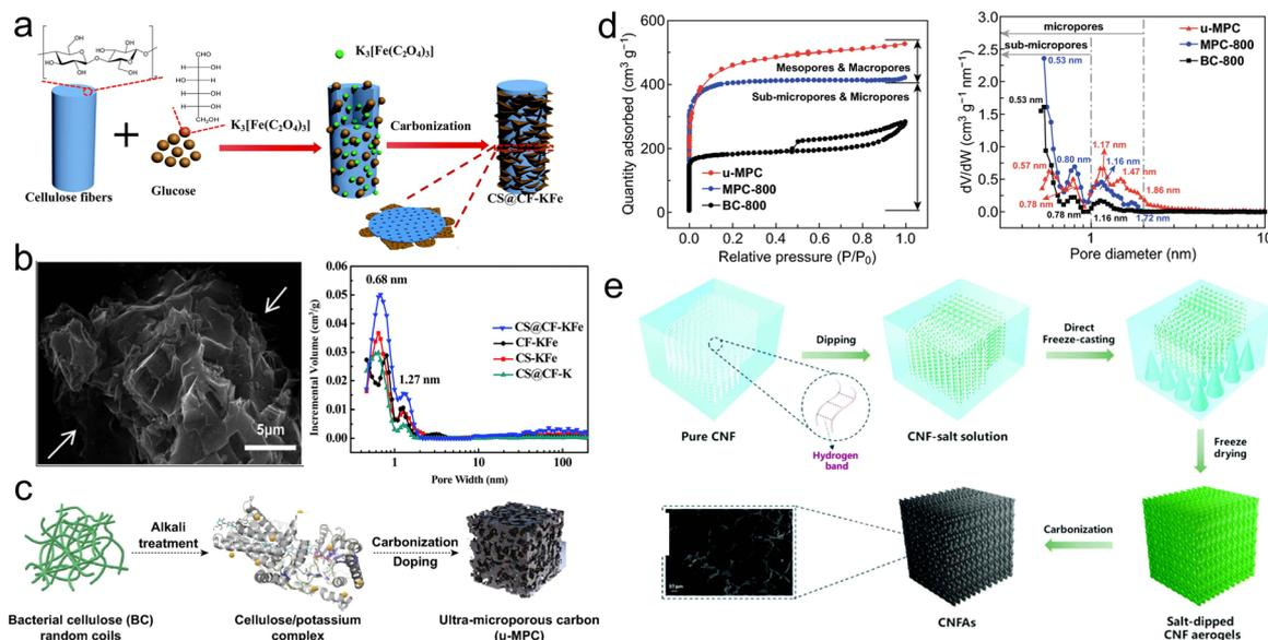
Fig. 2 (a) Synthetic route for the synthesis of CS@CF-KFe; (b) SEM and pore size distribution (PSD) plots of CS@CF-KFe;<sup>33</sup> (c) schematic for the synthesis of u-MPC; (d) nitrogen adsorption-desorption and PSD curves of samples;<sup>35</sup> (e) preparation process of CNFAs.<sup>36</sup>
