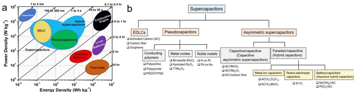
Fig. 1 (a) Ragone diagram of ESDs;<sup>23</sup> (b) classification of SCs and examples of corresponding electrode materials.<sup>5</sup>
