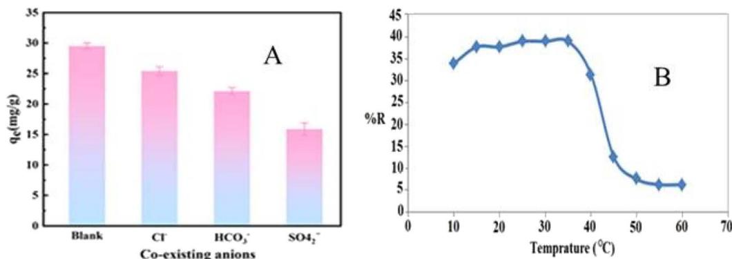
Fig. 9 (A) Effect of co-existing ions on  $\text{NO}_3^-$  adsorption onto GCS@LDH. Reproduced with permission from ref. 104 with permission from Elsevier, copyright 2022. (B) The temperature effect on the adsorption of  $\text{NO}_3^-$  onto CTS/ZY/ZrO<sub>2</sub> nanocomposite. Reproduced with permission from ref. 87 with permission from Elsevier, copyright 2016.
