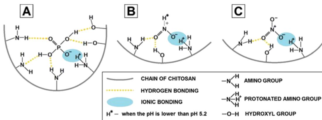
Fig. 7 Possible mechanisms of nutrient bonding onto chitosan sorbents: (A)  $\text{PO}_4^{3-}$ , (B)  $\text{N-NO}_2$ , and (C)  $\text{N-NO}_3$ . Reproduced with permission from ref. 92 with permission from Elsevier, copyright 2017.
