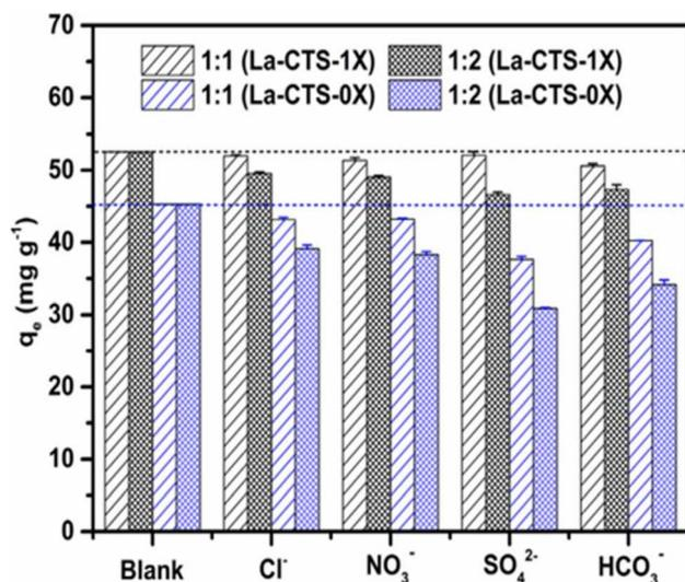
Fig. 4 Effect of coexisting ions on  $\text{PO}_4^{3-}$  recovery by La-CTS-1X and La-CTS-0X (the ratios of the initial  $\text{PO}_4^{3-}$  concentration to the coexisting ion concentration are 1 : 1 and 1 : 2). Reproduced with permission from ref. 96 with permission from Elsevier, copyright 2019.
