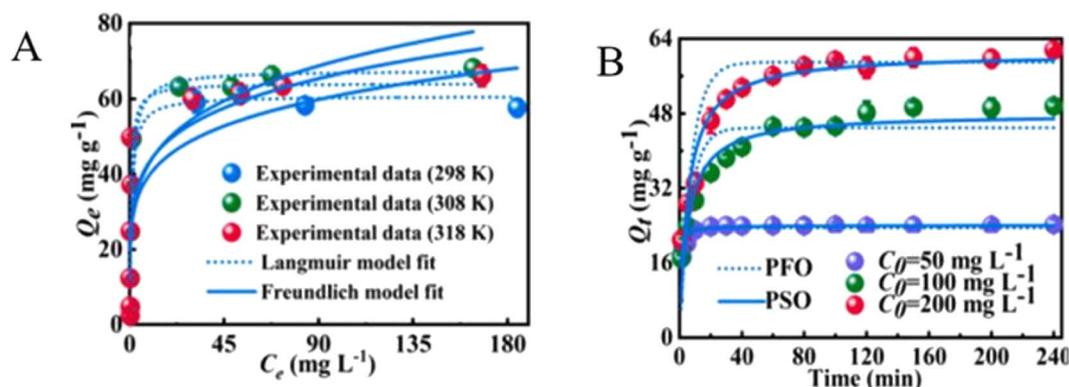
Fig. 6 (A) The Langmuir and Freundlich isotherm models and (B) pseudo-first-order and pseudo-second-order kinetics models for the adsorption of  $\text{PO}_4^{3-}$  on La/Fe-Cs composites. Reproduced with permission from ref. 1 with permission from Elsevier, copyright 2022.
