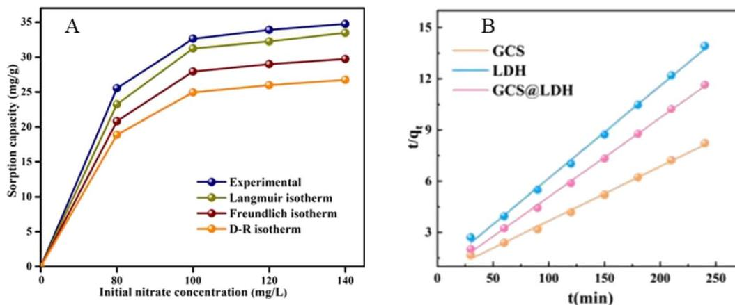
Fig. 11 (A) Experimentally measured isotherms for  $\text{NO}_3^-$  adsorption by Zr@AlgKN composite beads. Reproduced with permission from ref. 86 with permission from Elsevier, copyright 2020. (B) Pseudo-second-order model on  $\text{NO}_3^-$  removal by GCS, LDH, and GCS@LDH. Reproduced with permission from ref. 104 with permission from Elsevier, copyright 2022.
