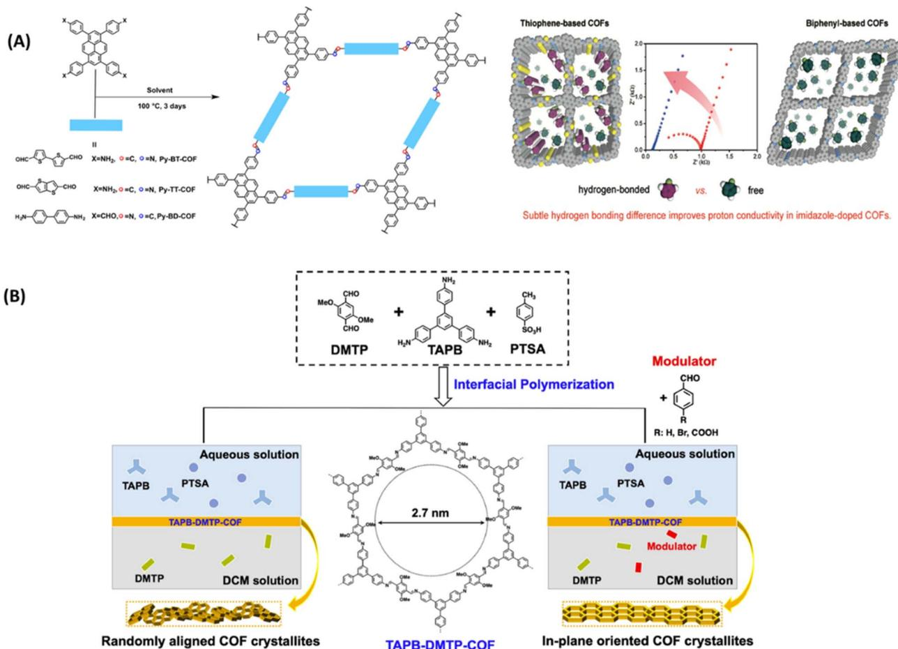
Fig. 12 (A) Synthesis of COFs and the demonstrated hydrogen bonding between doped imidazole with thiophene-based COFs. Reprinted with permission,<sup>65</sup> Copyright (2020) from American Chemical Society. (B) Synthesis of TAPB-DMTP-COF by interfacial polymerization. Reprinted with permission,<sup>66</sup> Copyright (2022) from Springer.
