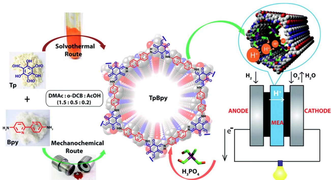
Fig. 3 Synthesis of TpBpy COF via solvothermal and mechanochemical routes, doping of  $\text{H}_3\text{PO}_4$  and their implementation in fuel cell as solid electrolyte. Reprinted with permission,<sup>51</sup> Copyright (2016) from Royal Society of Chemistry.
