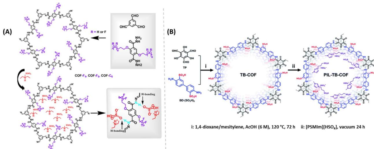
Fig. 11 (A) Synthesis of alkyl/perfluoroalkyl functionalized COFs doped with PILs and the hydrogen bond networks demonstrated. Reprinted with permission,<sup>63</sup> Copyright (2021) from American Chemical Society. (B) Synthesis of PIL doped TB-COF. Reprinted with permission,<sup>64</sup> Copyright (2022) from Royal Society of Chemistry.
