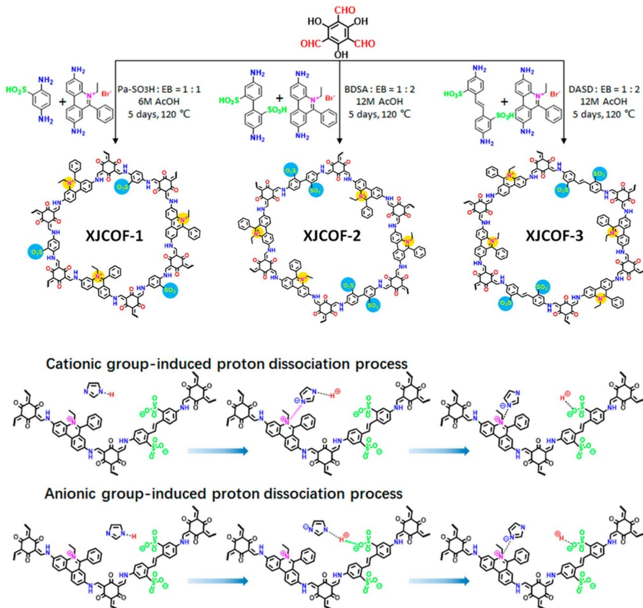
Fig. 14 Synthetic scheme of XJCOFs and the two possible processes for inducing proton dissociation in XJCOF-2 skeleton. Reprinted with permission,<sup>69</sup> Copyright (2021) from American Chemical Society.
