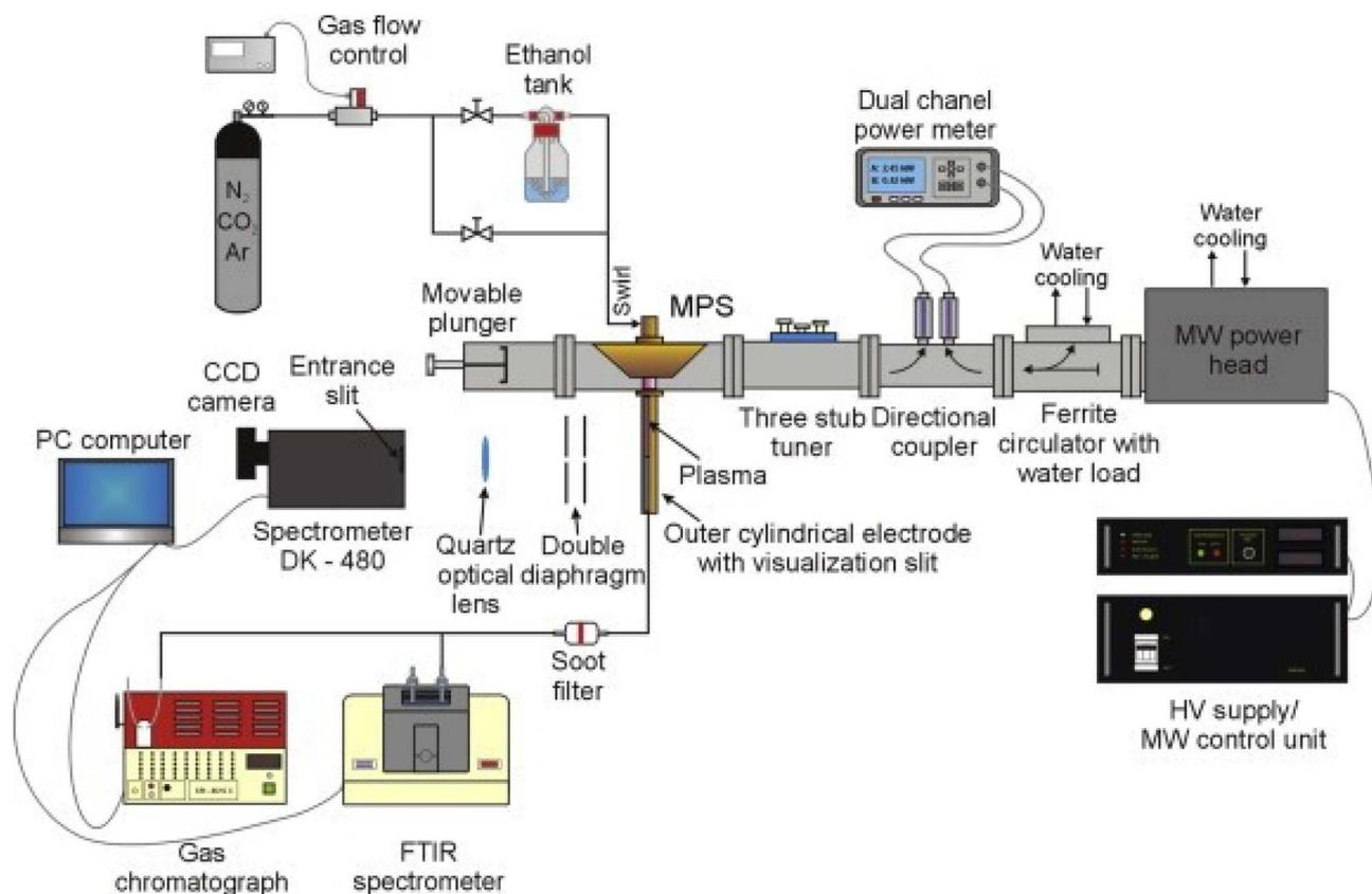
Fig. 2 Diagram of a microwave plasma hydrogen production system.<sup>110</sup>
