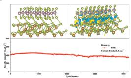
Self-assembled nanoflower-like FeSe<sub>2</sub>/MoSe<sub>2</sub> heterojunction anode with enhanced kinetics for superior-performance Na-ion half/full batteries
