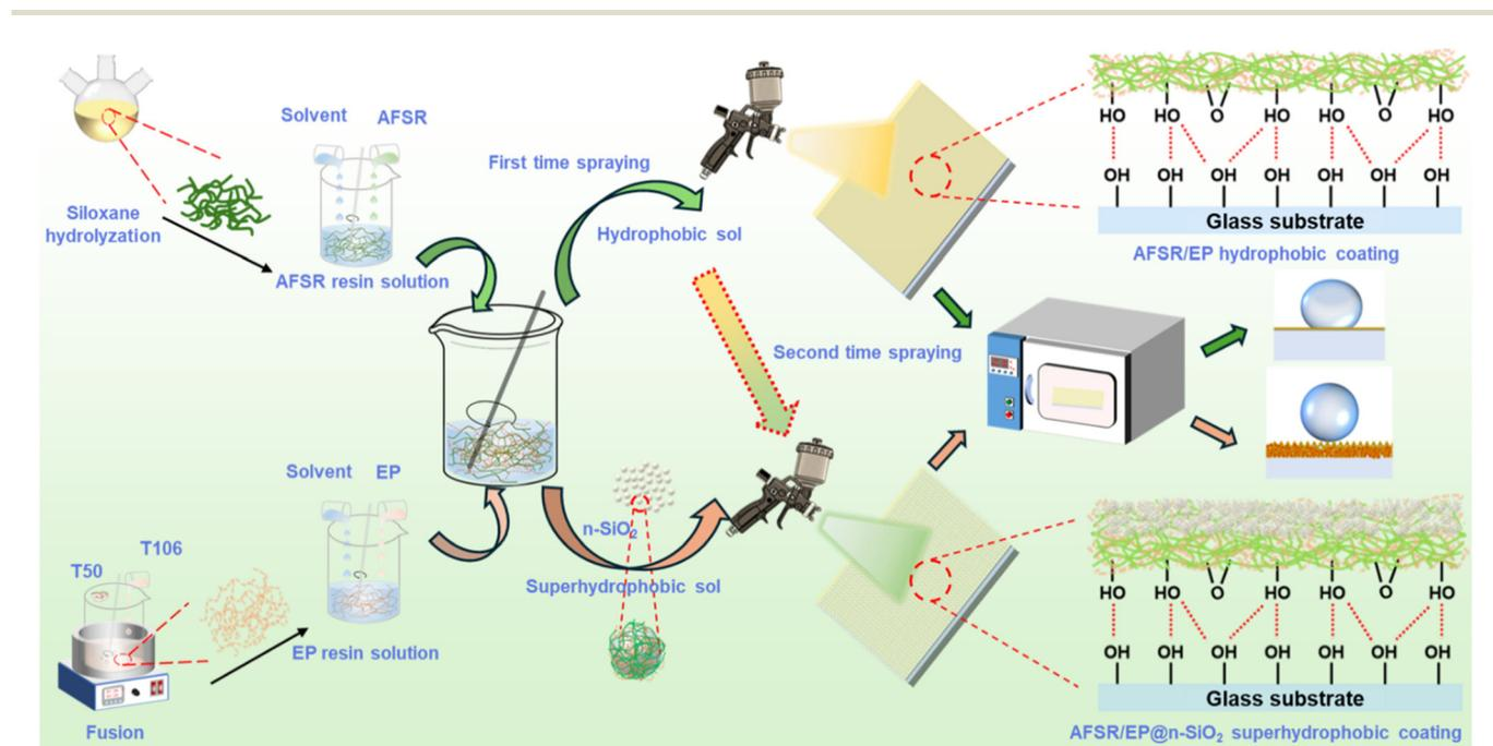
**Scheme 1** The fabrication process of AFSR/EP hydrophobic coating and AFSR/EP@n-SiO<sub>2</sub> superhydrophobic coating.
