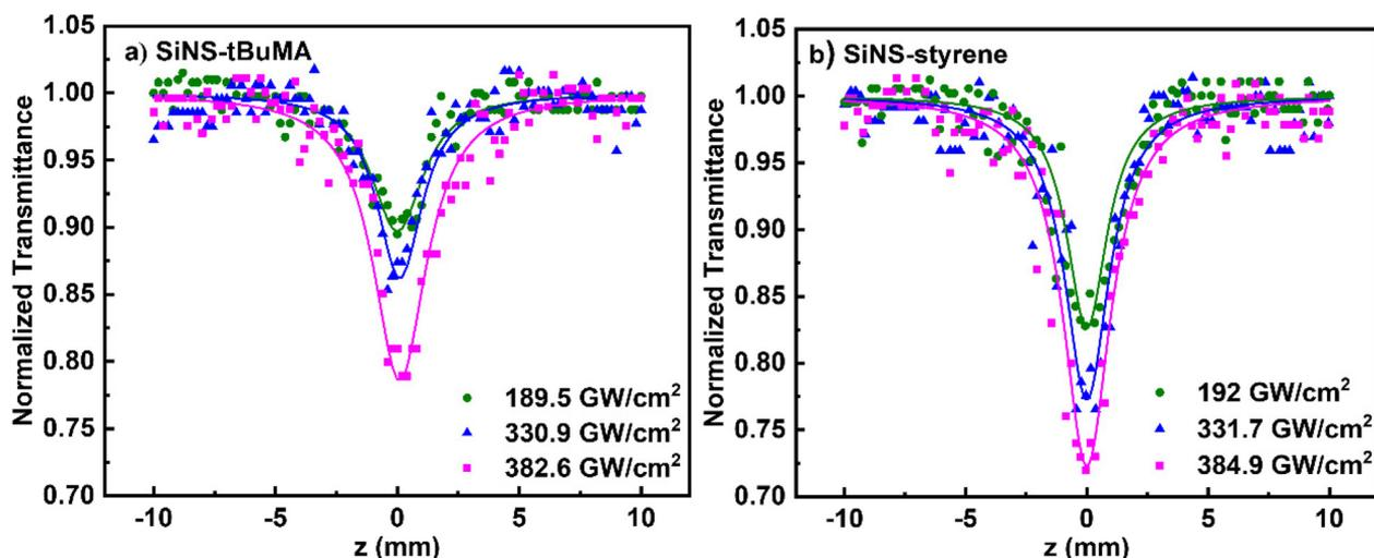
**Fig. 5** OA Z-scans of (a) SiNS-*t*BuMA and (b) SiNS-styrene dispersions under different laser intensities at 800 nm. All dispersions had a linear absorption coefficient  $\alpha_0$  of about  $1 \text{ cm}^{-1}$ .
