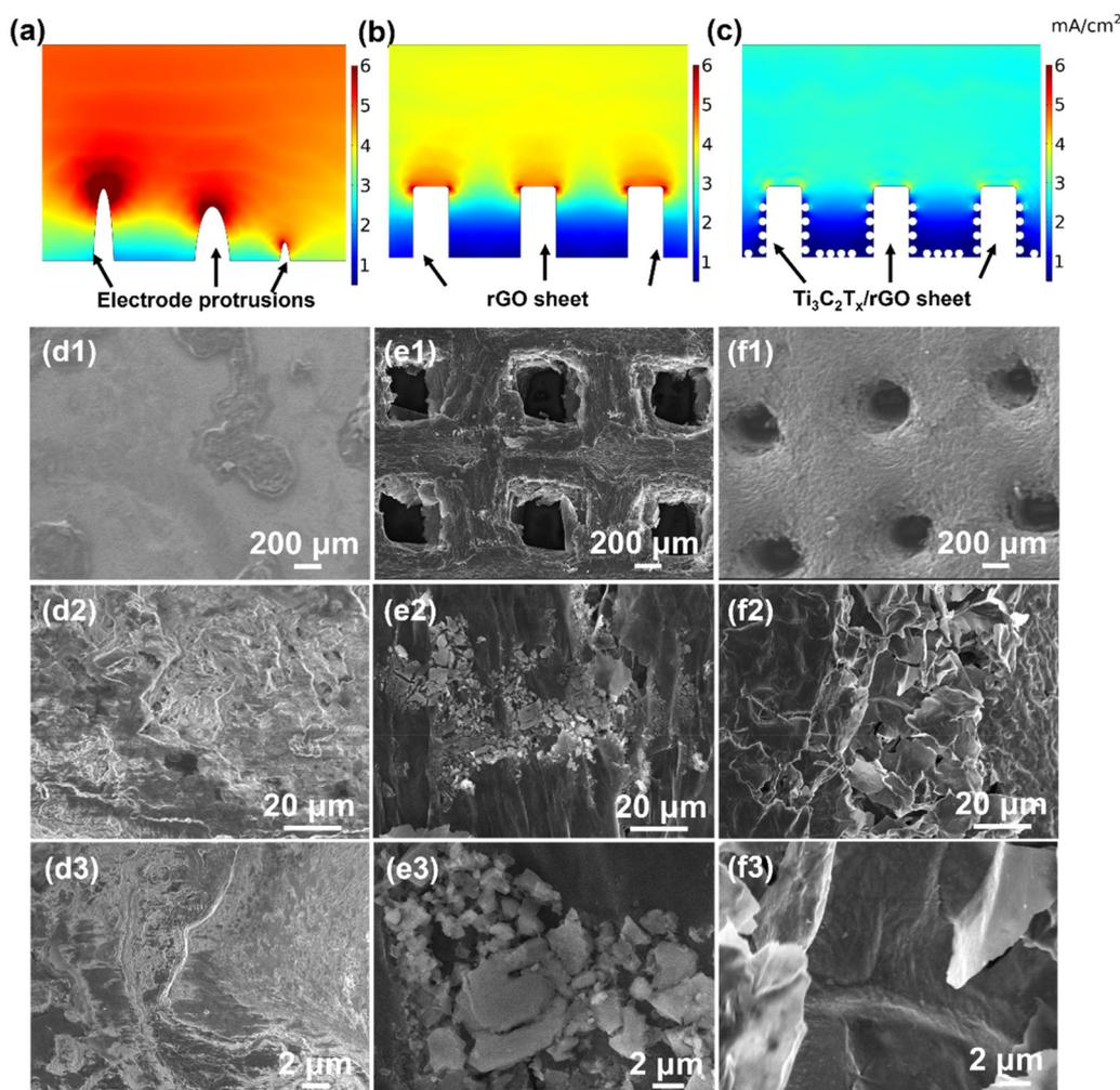
Fig. 4 Surface current density distribution simulated by COMSOL Multiphysics on (a) Cu, (b) 3D-printed rGO and (c) 3D-printed 50%  $Ti_3C_2T_x/rGO$  electrodes. SEM images of (d) Cu, (e) 3D-printed rGO and (f) 3D-printed 50%  $Ti_3C_2T_x/rGO$  electrodes after 100 cycles at  $2 \text{ mA cm}^{-2}$  with  $2 \text{ mA h cm}^{-2}$ .
