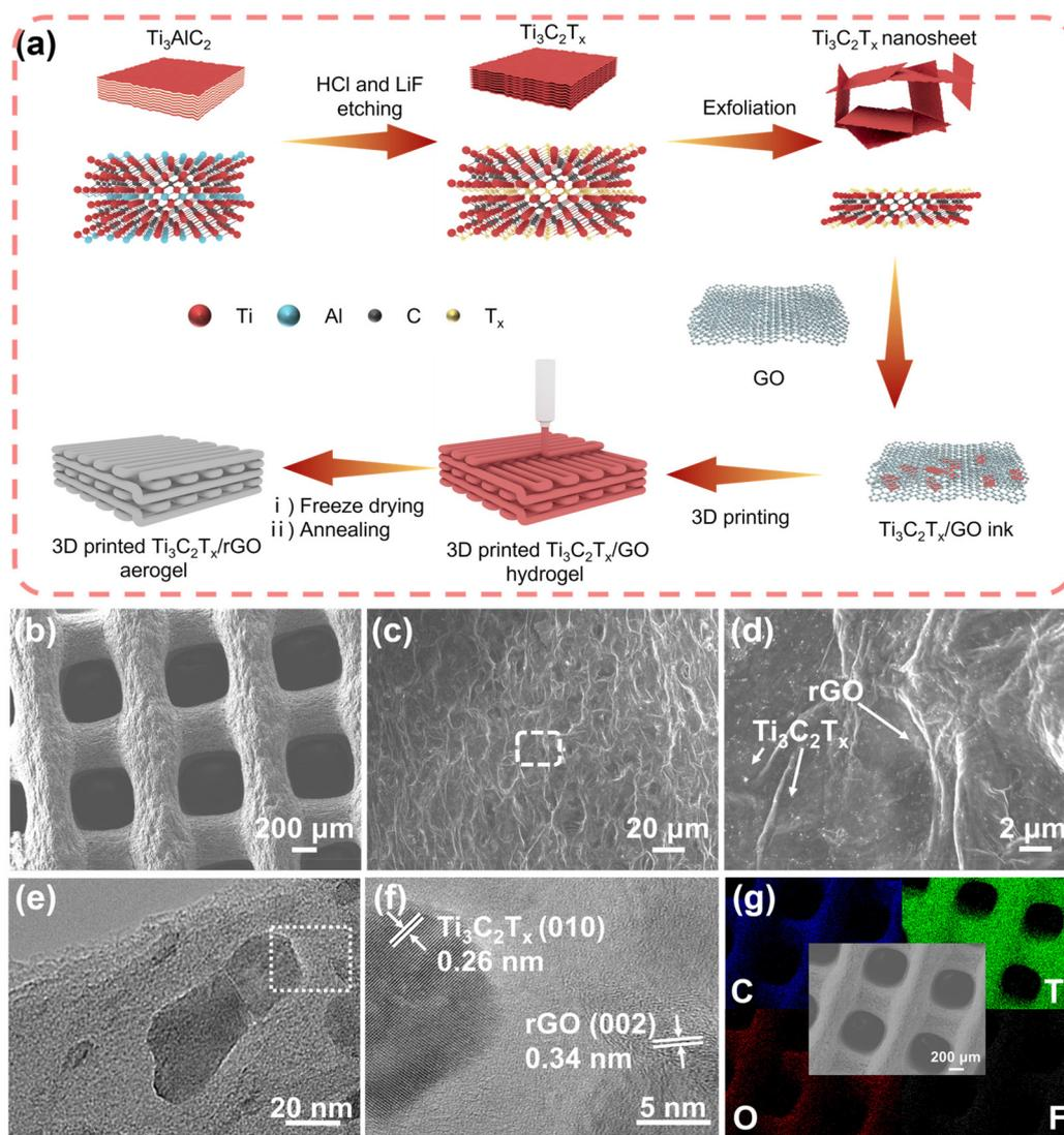
**Fig. 1** (a) A schematic diagram of the preparation process of 3D-printed  $\text{Ti}_3\text{C}_2\text{T}_x/\text{rGO}$  microlattice aerogel electrodes. (b–d) SEM and (e and f) TEM images of the 3D-printed 50%  $\text{Ti}_3\text{C}_2\text{T}_x/\text{rGO}$  electrode. (g) SEM image of the 3D-printed 50%  $\text{Ti}_3\text{C}_2\text{T}_x/\text{rGO}$  microlattice aerogel and the corresponding EDS elemental mapping.
