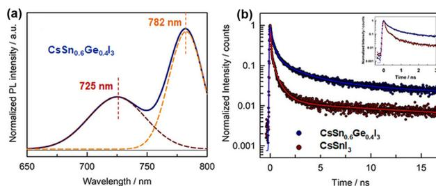
**Fig. 11** (a) Steady-state PL spectra of CsSn<sub>0.6</sub>Ge<sub>0.4</sub>I<sub>3</sub> NCs. (b) TRPL spectra of CsSn<sub>0.6</sub>Ge<sub>0.4</sub>I<sub>3</sub> and CsSnI<sub>3</sub>. Reproduced from ref. 86 with permission from Wiley-VCH, copyright 2020.
