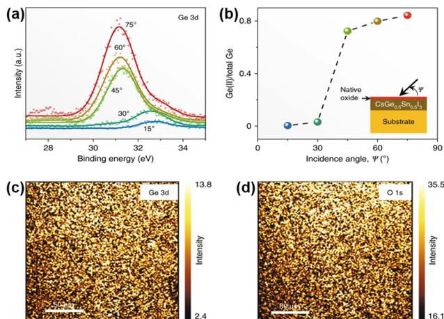
**Fig. 10** (a) Ge 3d XPS spectra at different incidence angles in a vapor-deposited CsSn<sub>0.5</sub>Ge<sub>0.5</sub>I<sub>3</sub> film. (b) The corresponding plot of the Ge(II) fraction vs. the incidence angle. (c) and (d) XPS maps of Ge 3d (33 eV) and O 1s (532 eV). Reproduced from ref. 82 with permission from Springer Nature. Copyright 2020.
