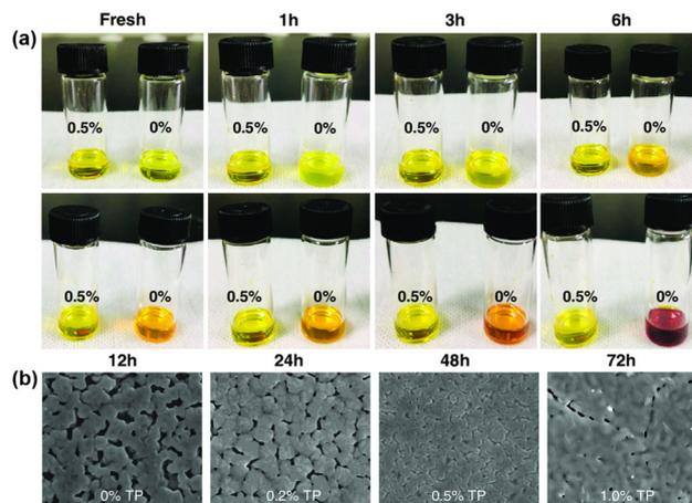
**Fig. 6** (a) Photographs of CsPb<sub>0.5</sub>Sn<sub>0.5</sub>I<sub>2</sub>Br precursor solutions with and without TP (0.5%). (b) Top-view SEM images of CsPb<sub>0.5</sub>Sn<sub>0.5</sub>I<sub>2</sub>Br thin films with varying TP contents. Reproduced from ref. 74 with permission from Wiley-VCH. Copyright 2020.
