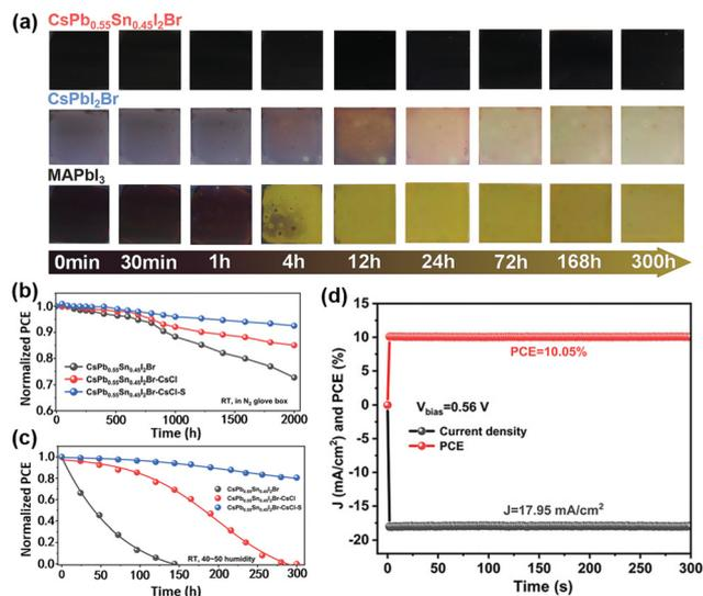
**Fig. 4** (a) Photographs of CsPb<sub>0.55</sub>Sn<sub>0.45</sub>I<sub>2</sub>Br, CsPbI<sub>2</sub>Br and MAPbI<sub>3</sub> perovskite films under iso-thermal annealing (150 °C) in an N<sub>2</sub>-filled glove box. The long-term normalized PCE of PSCs (b) in an N<sub>2</sub>-filled glovebox and (c) in the ambient air (40–50% RH). (d) MPPT of a CsPb<sub>0.55</sub>Sn<sub>0.45</sub>I<sub>2</sub>Br-CsCl-S-based device. Reproduced from ref. 68 with permission from Wiley-VCH. Copyright 2021.
