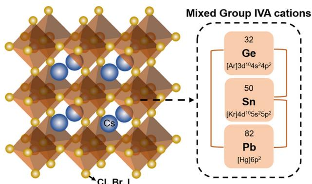
Fig. 1 Crystal structure of the all-inorganic ABX<sub>3</sub> perovskite based on mixed group IVA cations.
