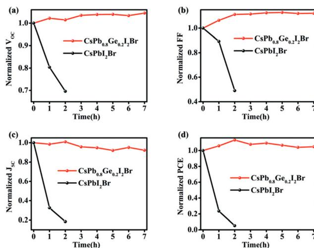
Fig. 8 Stability tests of CsPb<sub>0.8</sub>Ge<sub>0.2</sub>I<sub>2</sub>Br and CsPbI<sub>2</sub>Br PSCs upon the storage in the ambient atmosphere (50–60% RH): (a) V<sub>oc</sub>, (b) FF, (c) J<sub>sc</sub>, and (d) PCE. Reproduced from ref. 80 with permission from Wiley-VCH. Copyright 2018.
