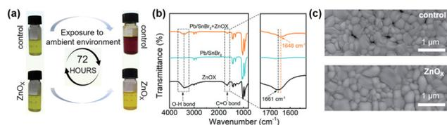
**Fig. 5** (a) Photographs confirming oxalate retarding the Sn<sup>2+</sup> oxidation. (b) FTIR spectra and the characteristic regions of pure ZnO<sub>x</sub>, Pb/SnBr<sub>2</sub>, and Pb/SnBr<sub>2</sub> + ZnO<sub>x</sub> in DMSO. (c) Top-view SEM images of CsPb<sub>0.7</sub>Sn<sub>0.3</sub>I<sub>2</sub>Br<sub>2</sub> thin films with and without ZnO<sub>x</sub>. Reproduced from ref. 67 with permission from Wiley-VCH, copyright 2022.
