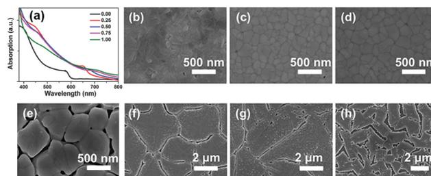
**Fig. 2** (a) UV-vis absorption spectra of  $\text{CsPb}_{1-x}\text{Sn}_x\text{I}\text{Br}_2$  with varying  $x$ . Reproduced from ref. 63 with permission from Wiley-VCH. Copyright 2018. Top-view SEM images of  $\text{CsPb}_{1-x}\text{Sn}_x\text{I}_3$  films with (b)  $x = 0$ , (c)  $x = 0.25$ , (d)  $x = 0.30$ , (e)  $x = 0.50$ , (f)  $x = 0.75$ , (g)  $x = 0.88$ , and (h)  $x = 1.00$ . Reproduced from ref. 64 with permission from the American Chemical Society. Copyright 2020.
