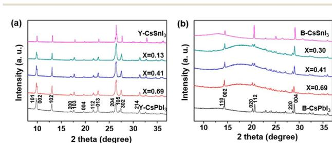
Fig. 7 XRD patterns of (a) Y-phase CsPb<sub>x</sub>Sn<sub>1-x</sub>I<sub>3</sub> NWs and (b) B-γ phase CsPb<sub>x</sub>Sn<sub>1-x</sub>I<sub>3</sub> NWs. Reproduced from ref. 78 with permission from the American Chemical Society. Copyright 2018.
