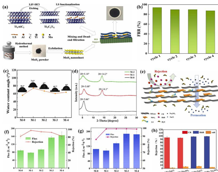
**Fig. 11** (a) Scheme for the preparation of  $\text{MoS}_2\text{@LS-MXene}$  composite films by pressure-assisted self-assembly. (b) FRR data of M-3. (c) CA of all membranes. (d) XRD patterns of M-0, M-1, and M-3. (e) Separation mechanism of  $\text{MoS}_2\text{@LS-MXene}$  composite membranes. Removal rates of dyes by different membranes: (f) CR and (g) RhB, and (h) separation of dye/salt mixture with M-3. Reprinted with permission.<sup>163</sup> Copyright 2022, Elsevier.
