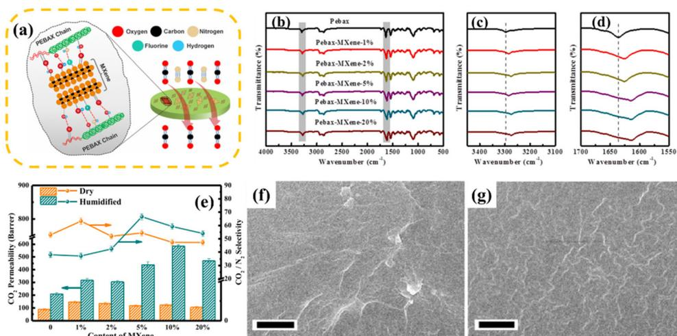
**Fig. 12** (a) Design of PeBax/MXene membrane. Reprinted with permission.<sup>85</sup> Copyright 2020, the American Chemical Society. (b)–(d) FTIR spectrum of PeBax-MXene films. (e) Gas transport characteristics of PeBax-MXene films under dry and wet conditions. (f) Cross sectional scanning electron microscopy images of PeBax-MXene-1% membrane and (g) PeBax-MXene-5% membrane. Reprinted with permission,<sup>169</sup> Copyright 2021, Elsevier.
