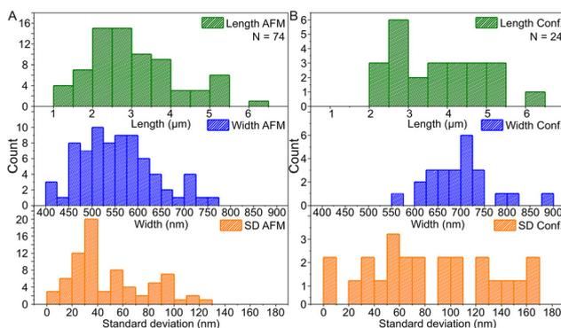
**Fig. 5** The histogram data of the dimensions of ribbons and tubes. (A) Histograms of the length, the width and the standard deviation of ribbon/tube width based on the AFM data and (B) the same histograms for the confocal microscopy data.  $N$  indicates the number of counted ribbons/tubes.
