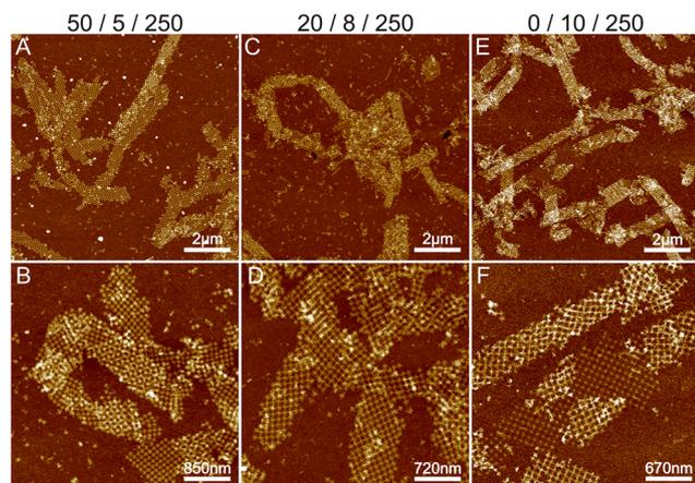
**Fig. 2** The effect of nickel on lattice formation. (A and B), (C and D) and (E and F) show AFM images of individual ST depositions when the concentrations  $C_{\text{Mg}^{2+}}/C_{\text{Ni}^{2+}}/C_{\text{Na}^+}$  are 50/5/250, 20/8/250 and 0/10/250 mM, respectively.
