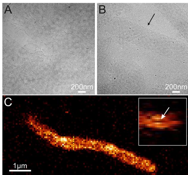
**Fig. 4** Cryo-TEM and confocal microscope images of different ribbons and tubes. (A) A cryo-TEM image of 2D ribbons, (B) a cryo-TEM image of 3D tubes and (C) a side view confocal microscope image of a 3D tube. The inset in C shows the cross-section highlighted by the yellow dashed line, where a small cavity can be seen inside the tube. The size of the inset is  $2 \mu\text{m} \times 2 \mu\text{m}$ .
