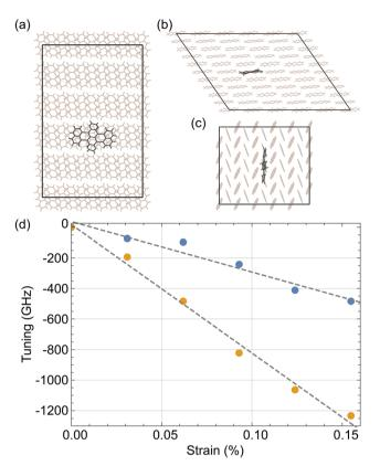
Fig. 5 (a)–(c) Projection of the  $5 \times 5 \times 3$  crystal cell that was used in our simulations on each of its a, b and c crystal axes. The DBT atoms are in the centre of the cell and are presented with grey colour. (d) Simulated detuning due to strain along the crystal's a (orange points) and b (blue points) axes and linear fittings in each of these cases (dashed grey lines).
