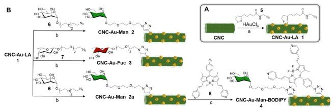
Scheme 1 A. Synthesis of CNC-Au-LA 1. B. Synthesis of CNC-Au-Man 2, CNC-Au-Fuc 3, and CNC-Au-Man-BODIPY 4. Reaction conditions: (a) NaBH<sub>4</sub>, MeOH: H<sub>2</sub>O (9:1), rt, 2 h; (b) CuSO<sub>4</sub>, sodium ascorbate, H<sub>2</sub>O, rt, 12 h; (c) CuSO<sub>4</sub>, sodium ascorbate, DMF, rt, 12 h.
