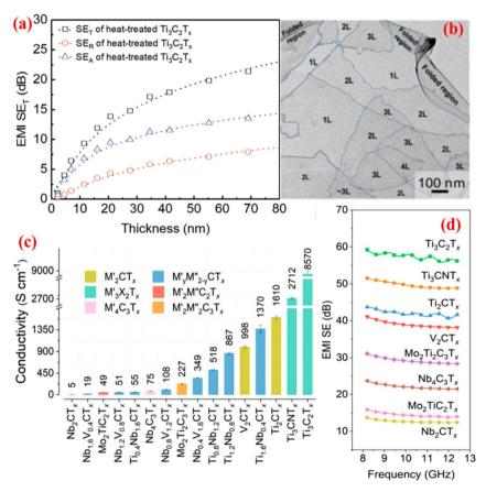
Fig. 2 (a) EMI SE values of  $T_{13}C_2T_x$  film after annealing at 400 °C and (b) transmission electron microscopy image of few-layer thick MXene film. Reproduced with permission from ref. 62 with permission from Wiley-VCH Verlag GmbH & Co. KGaA, Weinheim, © 2020. (c) Conductivity and (d) EMI SE of 5  $\mu$ m-thick MXene films with different compositions. Reproduced from ref. 63 with permission from the American Chemical Society, © 2020.
