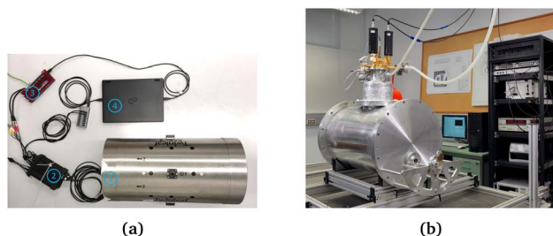
Fig. 3 (a) Tabletop TNM setup based on OPMs. The sample is placed inside the Twinleaf MS-2 shield (1) together with the two QZFM. QZFM electronics (2) control the sensors and a laptop (4) serves for driving the DAQ Labjack U6 (3) in stream mode, running the QZFM electronics and collecting the data. The sample is at an average distance of 13.5 mm from the gas cell with the polarized Rb atoms. (b) In-house developed SQUID setup for reference measurements. A superconducting Nb magnetic shield and 6 SQUID sensors are kept at LHe temperature; the sample is placed in a bore through the setup and kept at an average temperature of 43.0 \pm 0.5 °C to match the sample temperature in the tabletop setup. An average distance of 23.5 mm is measured between the pickup coils of the SQUID sensors and the sample. Only one sensor is used for the TNM measurement.
