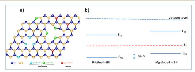
Fig. 5 (a) Proposed atomic arrangements of Mg impurities in h-BN of the three suggested Mg incorporation sites: graphitic, pyrrolic, and pyridinic. The crystal is viewed along the *c*-axis. (b) Band alignment and offset in our h-BN/graphene heterostructures, as determined from the ARPES data.
