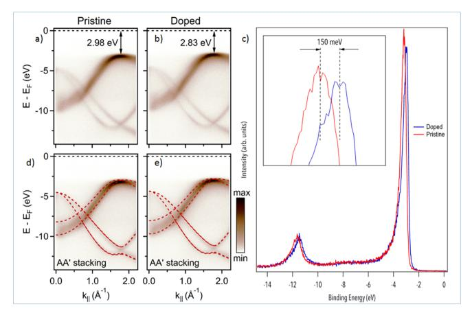
Fig. 3 Electronic structure of pristine and Mg doped h-BN: (a and b) nano-ARPES spectra of pristine h-BN and Mg-doped h-BN acquired at photon energy  $h\nu = 100$  eV, respectively. (c) Nano-ARPES intensity integrated spectra as a function of the binding energy, extracted from the 2D ARPES map, for pristine h-BN (red line) and Mg-doped h-BN (blue line). (d and e) Same nano-ARPES data with superposed band structure from DFT calculation (PBE) of bulk hexagonal AA' h-BN.
