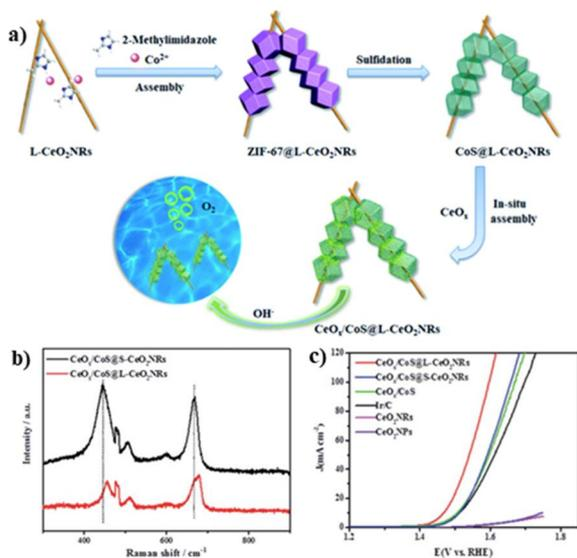
Fig. 2 (a) Scheme of the fabrication process of  $\text{CeO}_x/\text{CoS}@L\text{-CeO}_2\text{-NRs}$ ; (b) Raman spectra of  $\text{CeO}_x/\text{CoS}@L\text{-CeO}_2\text{-NRs}$  and  $\text{CeO}_x/\text{CoS}@S\text{-CeO}_2\text{-NRs}$ ; (c) LSV curves of different electrocatalysts. Reproduced with permission from ref. 63. © Royal Society of Chemistry, 2019.
