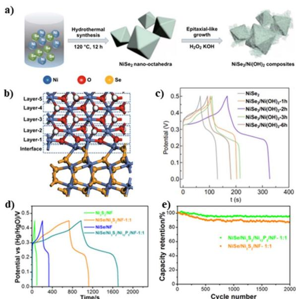
Fig. 6 (a) Synthetic process of the NiSe<sub>2</sub>/Ni(OH)<sub>2</sub> heterostructure; (b) cartoon of the heterointerface; (c) GCD curves of different catalysts; reproduced with permission from ref. 45. © Springer Nature, 2020. (d) GCD curves at 10 mA cm<sup>-2</sup> and (e) 2000 GCD cycles of the NiSe/Ni<sub>3</sub>S<sub>2</sub>/Ni<sub>12</sub>P<sub>5</sub> heterostructure and control samples. Reproduced with permission from ref. 42. © Elsevier, 2018.
