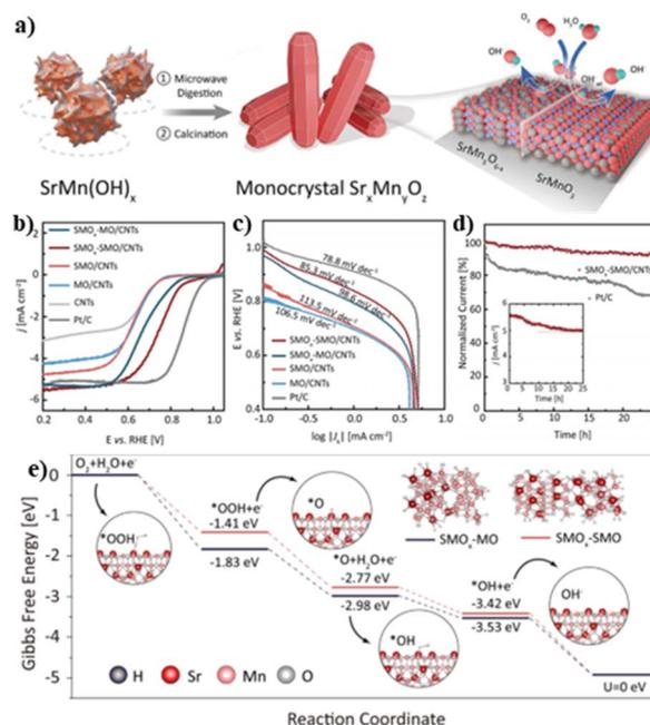
Fig. 5 (a) Scheme for the fabrication of SMO<sub>x</sub>-SMO; (b) LSV curves; (c) Tafel slopes and (d) chronoamperometric curves for different catalysts; (e) Gibbs free energy change chart for SMO<sub>x</sub>-SMO and SMO<sub>x</sub>-MO. Reproduced with permission from ref. 43. © Wiley-VCH GmbH, 2021.
