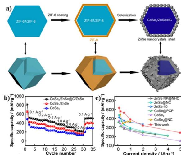
Fig. 9 (a) Synthetic process of CoSe<sub>2</sub>/ZnSe/NC@ZnSe/NC; (b) rate capacity of CoSe<sub>2</sub>/ZnSe/NC@ZnSe/NC, CoSe<sub>2</sub>/ZnSe and CoSe<sub>2</sub>; (c) comparison of rate capacity with other reported anode materials. Reproduced with permission from ref. 79. © Springer Nature, 2022.
