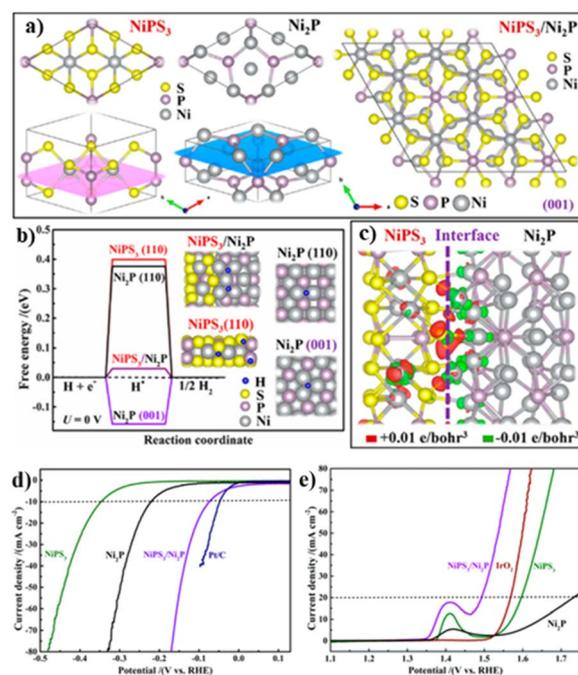
Fig. 3 (a) Graphical models to show the lattice match between  $\text{NiPS}_3$  and  $\text{Ni}_2\text{P}$ ; (b)  $\Delta G_{\text{H}^*}$  calculation; (c) charge density distribution at the interface, The Ni, S, P, and H atoms are marked in gray, yellow, purple, and blue, respectively; LSV curves of (d) HER and (e) OER. Reproduced with permission from ref. 44. © American Chemical Society, 2019.
