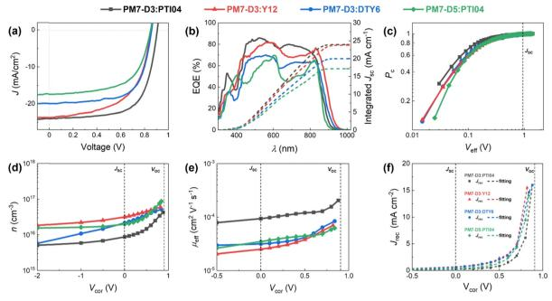
Fig. 2 (a) J-V characteristics, (b) EQE spectra, (c) charge collection probability, (d) voltage-dependent charge carrier density, (e) voltage-dependent effective mobility, and (f) fitting of the recombination current density of **PM7-D3:PTI04**, **PM7-D3:PTI04**, **PM7-D3:DTY6**, and **PM7-D5:PTI04** under AM1.5G illumination at 100 mW cm<sup>-2</sup>.
