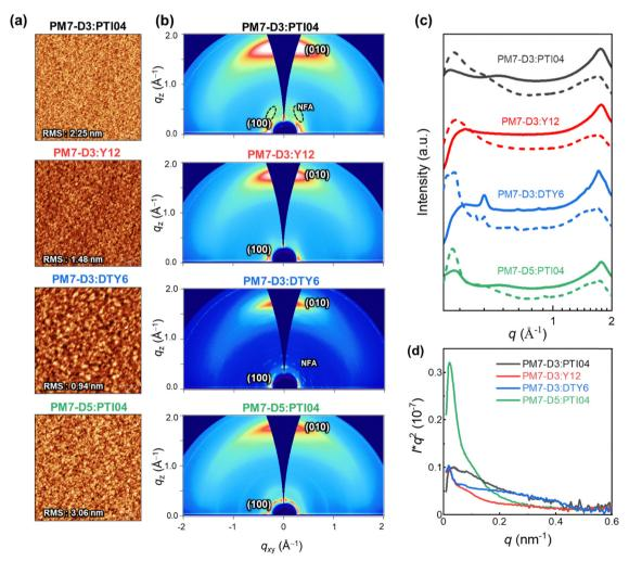
Fig. 3 Surface and bulk morphology of the BHJ blends processed from 2-MeTHF: (a) AFM topography images 5  $\mu$ m  $\times$  5  $\mu$ m, (b) 2D GIWAXS patterns, (c) the corresponding log-log plot of in-plane (dash lines) and out-of-plane (solid lines) GIWAXS profiles, and (d) RSoXS profiles at 285.0 eV with film thickness normalization and Lorentz correction.
