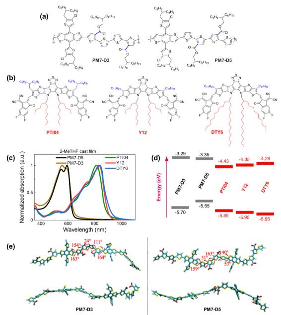
Fig. 1 Chemical structures of (a) PM7-D3 and PM7-D5, and (b) PTI04, Y12, and DTY6. (c) Normalized absorption of thin films processed from 2-MeTHF. (d) Energy level diagram of polymers donors and acceptors. (e) Top and side views of the optimized geometries (at the wB97X-D/6-31G(d,p) level of theory) for the symmetric dimeric models of PM7-D3 (left), and PM7-D5 (right) polymers. The dihedral angles between selected moieties are indicated in red. The long sidechains are omitted for clarity
