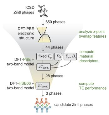
Fig. 4 Computational workflow to identify Zintl phases that are narrowgap semiconductors or semimetals and exhibit high room-temperature thermoelectric performance.  $E_g$  is the band gap,  $R_B$  is the asymmetry parameter, and  $B_{
