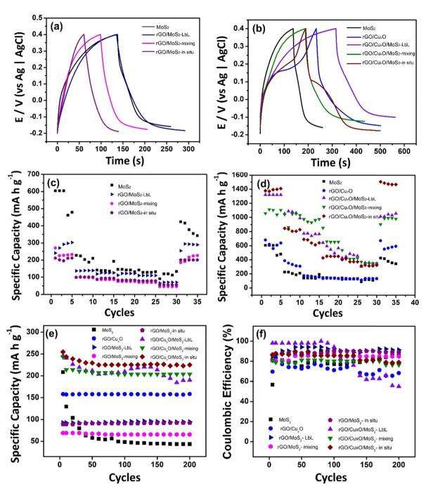
Fig. 8 Charge and discharge curves (a) and (b); specific capacity of the discharge process (c) and (d) at different current densities (0.1, 0.25, 0.5, 0.75, 1 and 2 A g<sup>-1</sup>); specific capacity measured during 200 cycles at 2 A g<sup>-1</sup> (e) and Coulombic efficiency (f) of the nanocomposites in 0.1 mol L<sup>-1</sup> NaCl aqueous solution and the potential range of -0.2 to 0.4 V.
