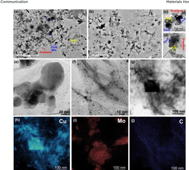
Fig. 5 Transmission electron microscopy images (a)-(g) and energy dispersive spectroscopy mapping images (h)-(j) of the rGO/Cu<sub>x</sub>O/ MoS<sub>2</sub>-in situ sample.
