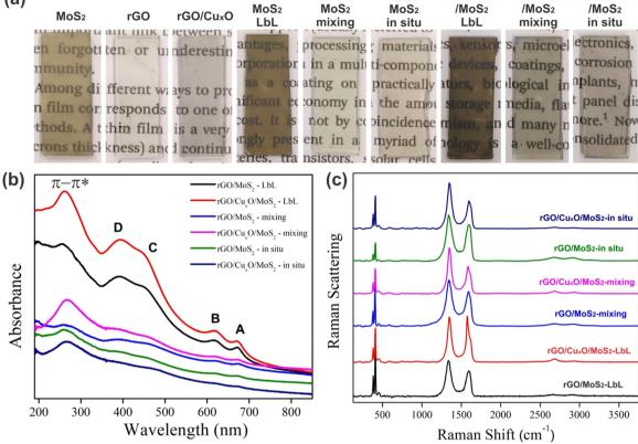
Fig. 2 Digital images of the films deposited over glass (a); UV-Vis (b) and Raman (c) (λ = 532 nm) spectra of the different nanocomposites
