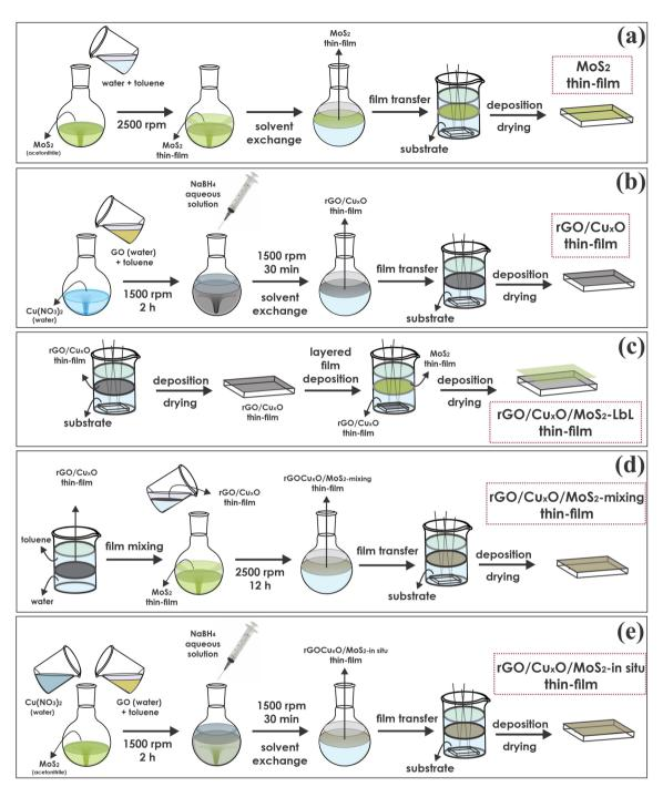
$\label{eq:fig.1} \textbf{Fig. 1} \quad \text{Schematic representation of the general steps for the thin film preparation: (a) $MoS_2$; (b) $rGO/Cu_xO$ or $rGO$; (c) $rGO/MoS_2$-LbL and $rGO/Cu_xO/MoS_2$-lbL; (d) $rGO/MoS_2$-mixing and $rGO/Cu_xO/MoS_2$-mixing; (e) $rGO/MoS_2$-in situ and $rGO/Cu_xO/MoS_2$-in situ.}$
