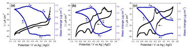
Fig. 7 Cyclic voltammograms (black) and evolution of the film mass (blue) during the third cycle (arrows indicate the scanning direction) for the  $MoS_2$  (a),  $rGO/Cu_xO$  (b) and  $rGO/Cu_xO/MoS_2$ -in situ (c) films. Conditions: Gold/quartz substrate, NaCl electrolyte (0.1 mol L<sup>-1</sup>) and scan rate 10 mV s<sup>-1</sup>.
