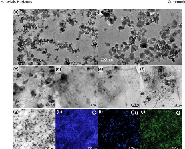
Fig. 4 Transmission electron microscopy images of the samples rGO/MoS<sub>2</sub> (a) and (b) and rGO/Cu<sub>x</sub>O (c)-(f). Energy dispersive spectroscopy mapping of  $rGO/Cu_xO(g)-(j)$ .
