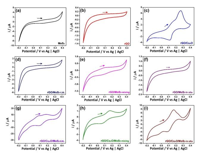
Fig. 6 Cyclic voltammograms of the thin films: (a) MoS<sub>2</sub>; (b) rGO; (c) rGO/Cu<sub>x</sub>O; (d) rGO/MoS<sub>2</sub>-LbL; (e) rGO/MoS<sub>2</sub>-mixing; (f) rGO/MoS<sub>2</sub>-in situ; (g) rGO/MoS<sub>2</sub>-th situ  $Cu_xO/MoS_2$ -LbL; (h)  $rGO/Cu_xO/MoS_2$ -mixing; (i)  $rGO/Cu_xO/MoS_2$ -in situ. Electrolyte: 0.1 mol L<sup>-1</sup> NaCl aqueous solution. Scan speed of 50 mV s<sup>-1</sup>
