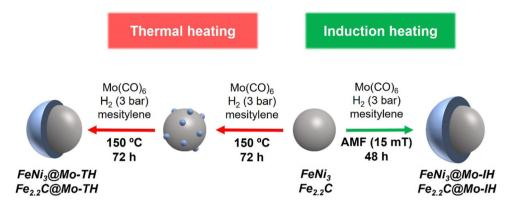
Scheme 1 Schematic representation of thermal and magnetically induced molybdenum coating on magnetic nanoparticles.
