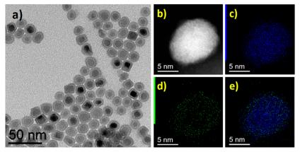
Fig. 2 Fe2.2C@Mo-TH NPs, (a) BF TEM image, (b) STEM-HAADF image and STEM-EDX mapping showing (c) Fe (blue), (d) Mo (green), and (e) overlap of Fe and Mo maps
