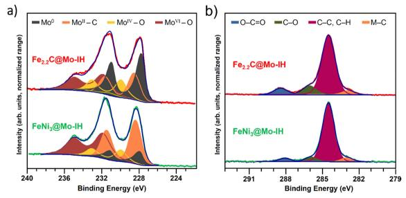
Fig. 5 (a) Mo3d and (b) C1s XPS regions for as-prepared core-shell nanoparticles assisted by induction heating after peak fitting. Note: doublet component colors are merged for a given chemical state for ease of visualization.
