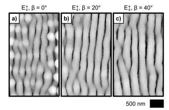
Fig. 3 Simulated deposit morphologies generated via growth modeling with vertically polarized (E  $\updownarrow$ )  $\lambda_{avg}$  = 626 nm illumination with the indicated inclination ( $\beta$ ) from the substrate normal in the plane of the polarization.
