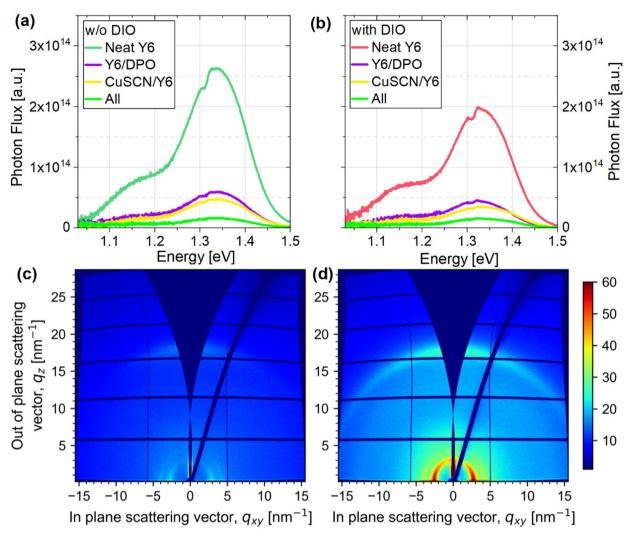
Fig. 3 Absolute photoluminescence spectra of the Y6 films with 15 nm thickness (a) without and (b) with DIO additive showing PL quenching when in contact with transport layers, measured in an integrating sphere. 2D GIWAXS images of (c) without and (d) with DIO Y6 films, where the q values are calculated with azimuthal integration.
