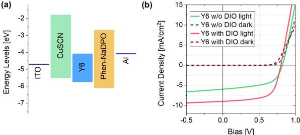
Fig. 1 (a) Energy levels (materials not in contact with each other) of the CuSCN<sup>21</sup> hole transport layer, small molecule acceptor Y6,<sup>22</sup> Phen-NaDPO<sup>23</sup> electron transport layer and of the electrodes  $^{21}$  taken from the literature. (b) Current density-voltage (J-V) characteristics of a regular device with a 100 nm neat Y6 active layer with and without the DIO additive measured under simulated AM1.5G light (solid lines) and in the dark (dashed lines).
