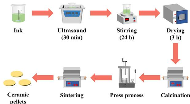
Fig. 1 Fabrication process of the doped GDC pellets.
