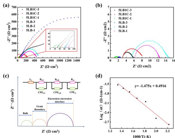
**Fig. 11** (a) Nyquist plots of 5LB1C and 5LB samples at 450 °C (The inset shows the enlarged view of high frequency part), (b) Nyquist plots of 5LB1C and 5LB samples at 750 °C, (c) illustration of a typical impedance plot for a polycrystalline sample with equivalent circuits, and (d) Arrhenius plot of the 5LB1C-1 sample.
