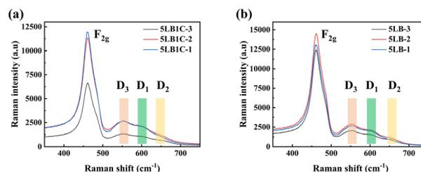
**Fig. 9** Raman spectra of 5LB1C and 5LB samples.
