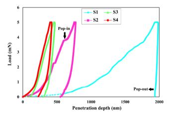
The load-displacement curves of the electrodeposited specimens.
