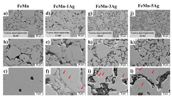
Fig. 2 SEM micrographs of sintered and surface-polished samples of FeMn (a-c), FeMn-1Ag (d-f), FeMn-3Ag (g-i) and FeMn-5Ag (j-l) samples. The % area macroporosity was determined using ImageJ by analyzing SEM images of the regions of macroporosity. The unlabeled red arrows provide reference for the Ag particles.
