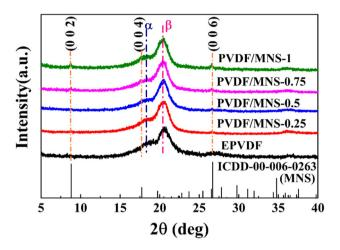
diffractograms of EPVDF and PVDF/MNS composite Fig. 7 X-ray nanofabrics
