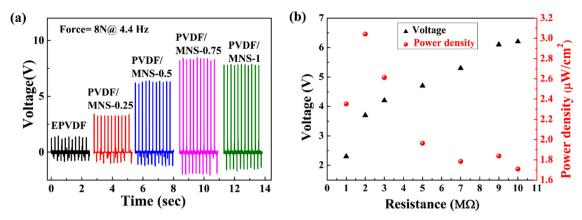
Fig. 11 (a) Piezoelectric response of EVPDF and PVDF/MNS composite nanofabrics-based PNG with varying loading of MNS, (b) piezoelectric voltage generated, and power density of PVDF/MNS-0.75 based PNG across the different resistances (applied force of 8 N).
