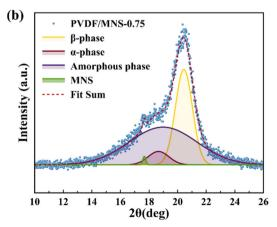
Fig. 8 Deconvoluted X-ray diffractograms of (a) EPVDF and (b) PVDF/MNS-0.75.
