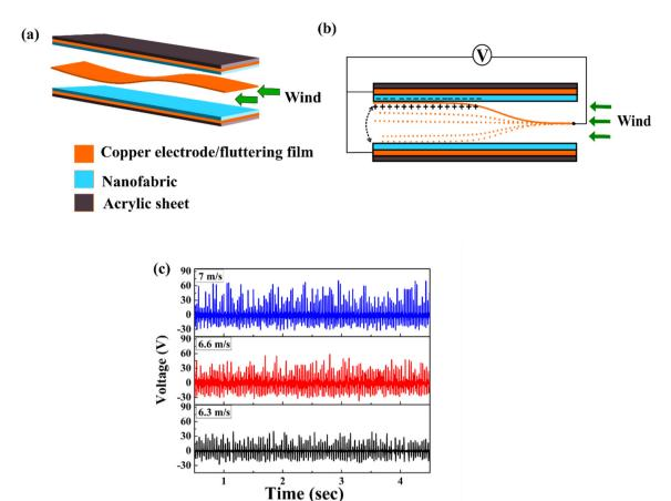
Fig. 13 (a) Schematic of the FL-TENG, (b) schematic of the working mechanism of FL-TENG, and (c) triboelectric performance of PVDF/MNS-0.75 based FL-TENG when exposed to varying wind speeds.
