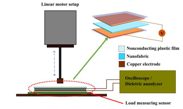
Fig. 1 Schematic of the piezoelectric/piezo capacitance measurement setup.
