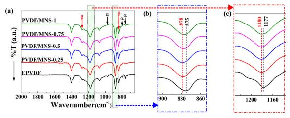
Fig. 5 FTIR spectra of EPVDF and PVDF/MNS composite nanofabrics (a)  $2000-650 \text{ cm}^{-1}$ , (b)  $900-860 \text{ cm}^{-1}$ , (c)  $1230-1140 \text{ cm}^{-1}$ .
