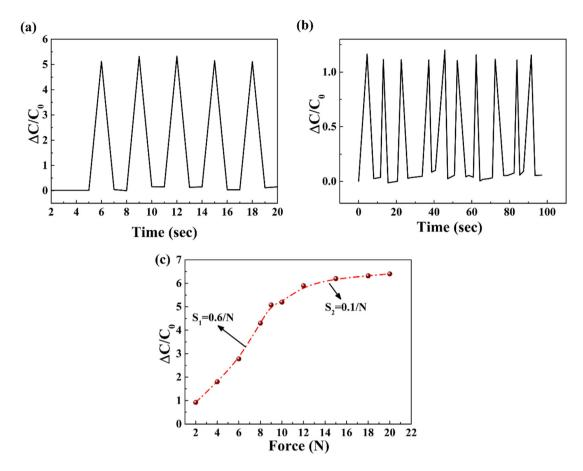
Fig. 10 (a) The response  $(\Delta C/C_0)$  of PVDF/MNS-0.75 based capacitive sensor (under 9 N load), (b) the response  $(\Delta C/C_0)$  of EPVDF based capacitive sensor (under 9 N load), and (c) ratio of relative change in capacitance to the initial capacitance of the sensor as a function of the applied load.
