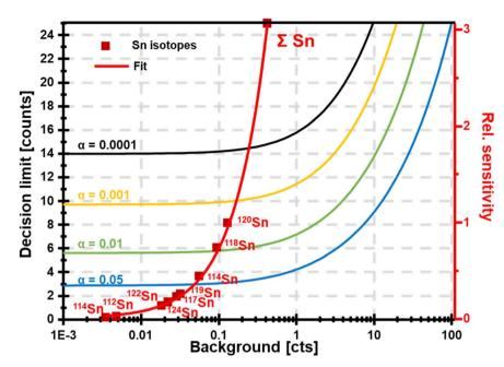
Fig. 6 Sensitivity is dependent on the fraction of Sn analysed. Considering abundant Sn isotopes or the sum of Sn isotopes increases sensitivity. However, concomitantly, decision limits increase due to increasing background signals. It is visible that sensitivity grows more rapidly than decision limits, which provides the opportunity to enhance detection limits through the bandpass mode.
