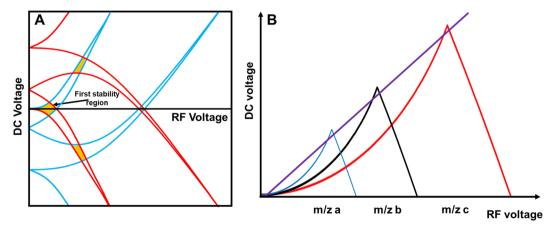
Fig. 1 (A) Shows the Matthieu stability plot for one m/z. (B) Shows the first stability region for three different m/z.
