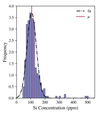
Fig. 3 Silicon concentration distribution in woody pellets (n=300 samples) as measured with the LIBS calibration model. Genotypes can be ranked as having low, medium, high, or very high silicon contents based on where they fall relative to the population.
