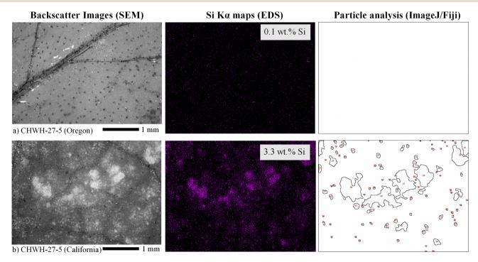
Fig. 6 Backscattered electron images from SEM, silicon  $K_{\alpha}$  maps from EDS, and particle analysis images of leaf areas (30× magnification) from genotype CHWH-27-5 collected from either (a) Oregon or (b) California. The leaf area shown in panel (a) has a very low silicon concentration (0.1 wt%) and no identifiable phytoliths. The leaf area shown in panel (b) has a moderate silicon concentration and phytolith abundance.
