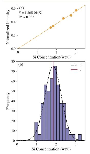
Fig. 4 (a) Silicon calibration model for leaf pellets built through the same standard addition process as that described for the woody pellets, and (b) distribution of silicon concentrations in leaf pellet samples as measured with LIBS calibration model.
