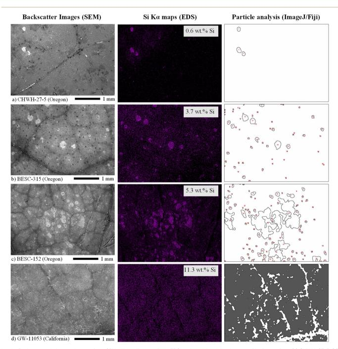
Fig. 7 Backscattered electron images from SEM, silicon  $K_{\alpha}$  maps from EDS, and particle outline images of leaf areas from (a) CHWH-27-5, (b) BESC-315, (c) BESC-152, and (d) GW-11053 genotypes, representing a large range of silicon concentrations. The genotype and collection site of each leaf are labeled on each SEM image, which have been slightly cropped at the bottom. The high-silicon part of the particle analysis image of (d) is represented by the gray area.
