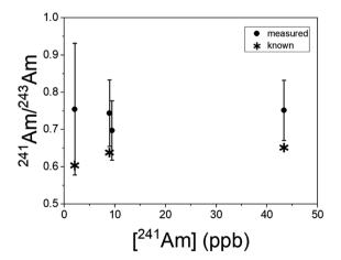
Fig. 6 241Am/243Am isotope ratios in BCR-2x samples as a function of the <sup>241</sup>Am concentration. Repeated measurements are slightly offset from one another in concentration for clarity. The asterisks correspond to ratios calculated from the composition of the Am standard plus  $^{241}$ Am in growth from the Pu standard. Uncertainties are  $1\sigma$
