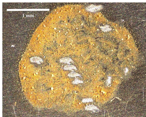
Fig. 2 Optical micrograph of sample BCR-2B deposited on a Ti metal substrate. The desorption laser spots from multiple analyses are clearly visible.
