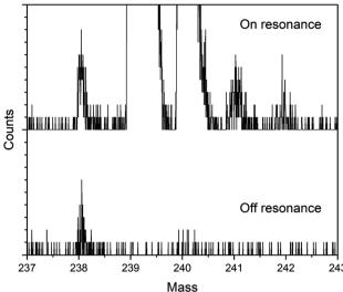
Fig. 3 On-resonance (upper) and off-resonance (lower) Pu RIMS spectra of sample BCR-2B. The  $^{238}$ Pu concentration is 0.47 ppb and the  $^{238}$ U/ $^{238}$ Pu ratio is 2.2  $\times$  10<sup>4</sup>. Each tick mark on the *y*-axis corresponds to a single ion count.
