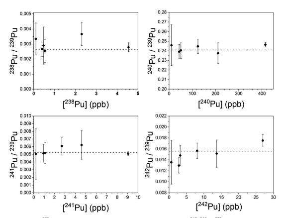
Fig. 7 Pu isotope ratios ( $^{8}$ Pu/ $^{239}$ Pu) as a function of the concentration of the minor isotope.  $^{240-242}$ Pu/ $^{239}$ Pu was measured by the simultaneous method;  $^{238}$ Pu/ $^{239}$ Pu was measured by the blinking method. Dashed lines are the certified ratios. Repeated measurements are slightly offset from one another in concentration for clarity. Uncertainties are  $1\sigma$ .
