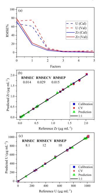
Fig. 2 Plot of (a) RMSE% *versus* the number of factors, (b) Zr parity plot with RMSE values, and (c) U parity plot with RMSE values. RMSE values are in parts per million ( $\mu$ g mL<sup>-1</sup>).
