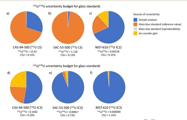
Fig. 2 Uranium isotope ratio uncertainty budgets for the three glass standards. The uncertainty budgets for  $^{235}$ U/ $^{238}$ U are provided in (a–c) and uncertainty budgets for  $^{234}$ U/ $^{238}$ U are provided in (d–f).
