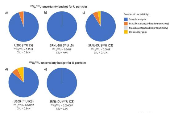
Fig. 8 Uranium isotope uncertainty budgets for the two U particle standards. The uncertainty budgets for  $^{235}$ U/ $^{238}$ U are provided in (a–c) and uncertainty budgets for  $^{234}$ U/ $^{238}$ U are provided in (d) and (e). The  $^{234}$ U/ $^{238}$ U uncertainty budget is largely representative of the budget for  $^{236}$ U/ $^{238}$ U.
