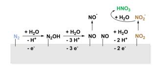
Fig. 6 Electrochemical activation of  $N_2$  via surface bound \*N<sub>2</sub>OH and \*NO to yield  $NO_2$ .
