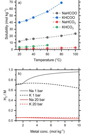
(a) Solubilities of Na and K salts; (b) equilibrium conversion, expressed as the molar ratio of H<sub>2</sub> gas to metal, of aqueous Na and K formate/bicarbonate solutions between 1 and 10 mol  ${
