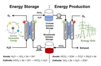
Fig. 8 Conceptual depiction of the electrochemical formate-bicarbonate cycle to store and to release energy. This approach does not require gaseous  $H_2$ .
