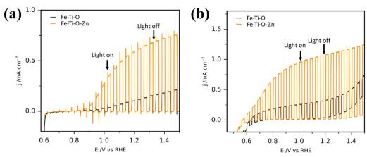
Fig. 12 Photocurrent density plots for Fe<sub>2</sub>TiO<sub>5</sub> and Zn-doped Fe<sub>2</sub>TiO<sub>5</sub> photoanodes (a) without hole quencher present, (b) with 10% H<sub>2</sub>O<sub>2</sub> in the solution. Reproduced with permission from ref. 179 copyright 2020, American Chemical Society.
