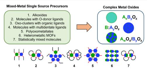
Fig. 21 Structures for mixed-metal SSPs and the deposited complex metal oxides. Reproduced with permission from ref. 261 copyright 2020, Royal Society of Chemistry
