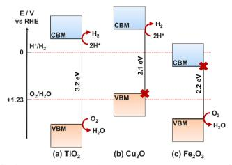
Fig. 4 Bandgap energy levels for three semiconductor examples at pH 0 relative to HER and OER redox potentials. (a) TiO<sub>2</sub> electrode: both HER and OER allowed, (b) Cu<sub>2</sub>O electrode: HER allowed, OER forbidden, (c) Fe<sub>2</sub>O<sub>3</sub> electrode: HER forbidden, OER allowed
