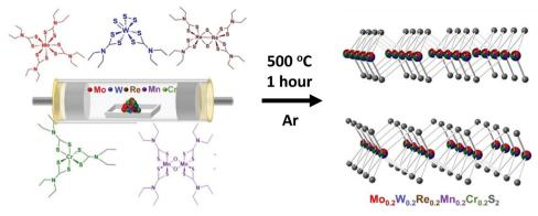
Fig. 33 Schematic of the preparation of a high entropy transition metal disulfide by the thermal decomposition of five precursor powders in tandem. Reproduced with permission from ref. 350 copyright 2023, Wiley-VCH.
