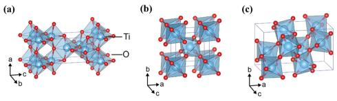
Fig. 7 Crystalline structures of TiO2 in polymorphs (a) anatase, (b) rutile, (c) brookite. Reproduced with permission from ref. 76 copyright 2017, Nature Portfolio
