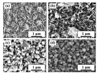
Fig. 17 Scanning electron micrographs of  $TiO_2$  grown on steel substrate by AACVD use carrier solvent of (a) ethanol, (b) methanol, (c) 10% methanol and 90% ethanol, (d) 25% methanol and 75% ethanol. Reproduced with permission from ref. 217 copyright 2012, Wiley-VCH.
