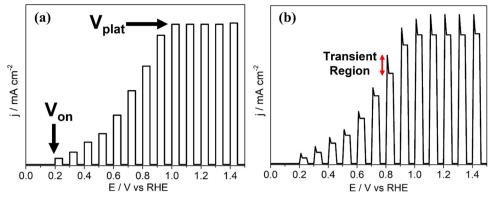
Fig. 6 Photocurrent density (j-V) graphs for example systems under chopped light showing (a) onset potential,  $V_{\text{ont}}$  and plateau potential,  $V_{\text{plate}}$  (b) photocurrent transients
