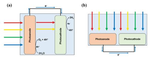
Fig. 3 Schematics showing PEC setups for (a) conventional tandem and (b) parallel configurations.
