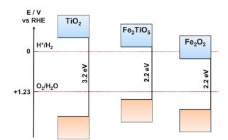
Fig. 9 Band positions for  $TiO_2$ ,  $\alpha$ -Fe<sub>2</sub>O<sub>3</sub>, and Fe<sub>2</sub>TiO<sub>5</sub>
