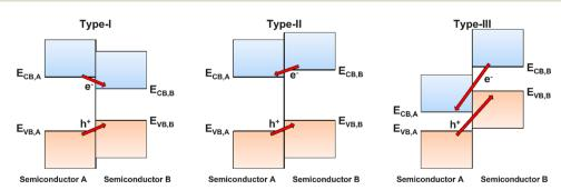
Fig. 29 Variations of heterojunction based on energy band alignments
