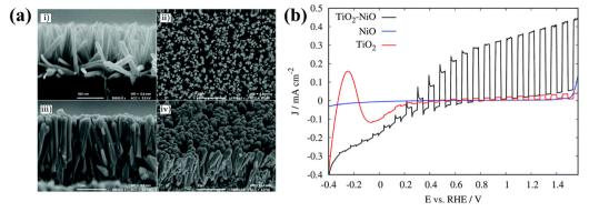
Fig. 30 (a) Scanning electron microscopy images of TiO<sub>2</sub> nanorods before (above) and after (below) NiO ALD coating, (b) photocurrent densities measured under chopped 1 sun rear-side illumination for TiO2, NiO, and NiO-coated TiO2 systems. Reproduced with permission from ref. 327 copyright 2021, Royal Society of Chemistry
