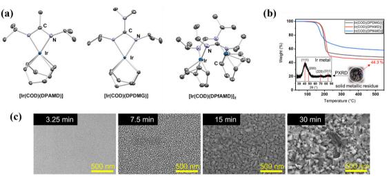
Fig. 31 (a) Structures of three bespoke Ir precursors, (b) TGA curves for the three complexes with PXRD of the residue for [Ir(COD)(DPAMD)], (c) SEM images of the Ir film deposited from [Ir(COD)(DPAMD)] with varying deposition times. Reproduced with permission from ref. 339 copyright 2022, American Chemical Society.
