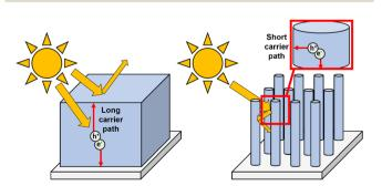
Fig. 11 Schematic comparisons of light trapping and carrier diffusion distances in a flat film versus nanorods
