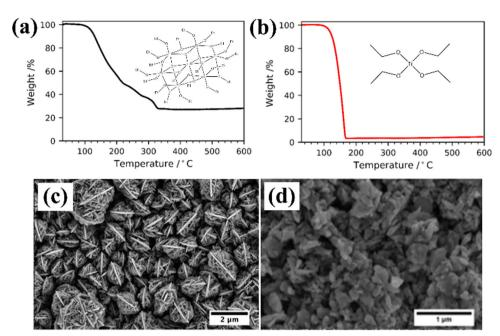
Fig. 25 Thermogravimetric analysis data for (a) [Ti<sub>7</sub>O<sub>4</sub>(OEt)<sub>20</sub>], (b) [Ti(OEt)<sub>4</sub>], inserts show the respective molecular structures; and SEM micrographs of films deposited using 0.35 M concentration of precursors (c) [Ti<sub>7</sub>O<sub>4</sub>(OEt)<sub>20</sub>], (d) [Ti(OEt)<sub>4</sub>]. Reproduced with permission from ref. 139 copyright 2019, Royal Society of Chemistry.
