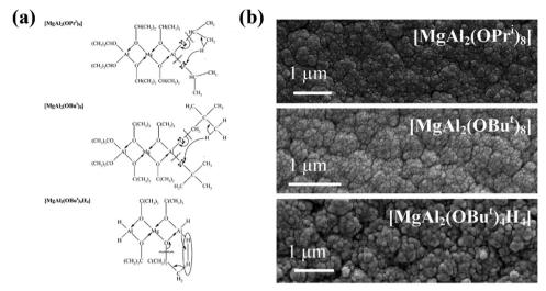
Fig. 16 (a) Proposed decomposition methods and (b) scanning electron microscopy surface images for precursors (top to bottom) [MgAl<sub>2</sub>(O<sup>i</sup>Pr)<sub>8</sub>], [MgAl<sub>2</sub>(O<sup>i</sup>Pr)<sub>8</sub>], [MgAl<sub>2</sub>(O<sup>i</sup>Pr)<sub>8</sub>]. Reproduced with permission from ref. 204 copyright 2004, American Chemical Society
