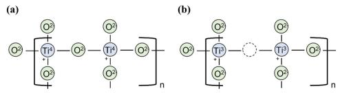
Fig. 8 (a) Defect free rutile  $TiO_2$ . (b) Intrinsic oxygen vacancy in rutile  $TiO_2$  causing reduction of  $Ti^{4+}$  to  $Ti^{3+}$  in the lattice to conserve overall charge neutrality
