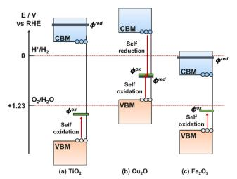
Fig. 15 Band energy levels for three common semiconductors compared to their reduction potentials ( $\varphi^{\text{ox}}$ , grey) and oxidation potentials ( $\varphi^{\text{red}}$ , green).
