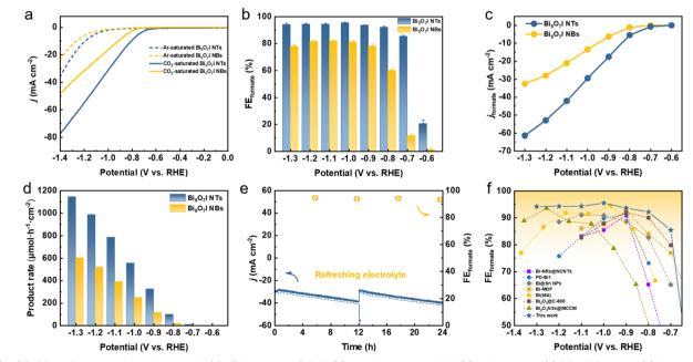
Fig. 2  $CO_2RR$  performance in a H-type cell. (a) LSV curves in 0.5 M  $CO_2$ - or Ar-saturated KHCO3 electrolyte, (b) FEs of formate, (c)  $j_{formate}$  and (d) formate formation rates of Bi<sub>5</sub>O<sub>7</sub>I NTs and NBs; (e) stability test of Bi<sub>5</sub>O<sub>7</sub>I NTs at -1.0 V in 0.5 M CO<sub>2</sub>-saturated KHCO<sub>3</sub> electrolyte; (f) comparison of FE<sub>formate</sub> of this work with recently reported Bi-based catalysts.
