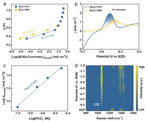
Fig. 4 Kinetic and mechanistic studies. (a) ECSA-corrected Tafel plots for formate production, (b) oxidative LSV curves in  $N_2$ -saturated 0.1 M KOH, (c)  $j_{formate}$  of  $Bi_5O_7l$  NTs in different concentrations of  $HCO_3^-$  at -1.0 V vs. RHE, and (d) potential-dependent Raman spectra on  $Bi_5O_7l$  NTs in 0.5 M  $CO_2$ -saturated KHCO3.
