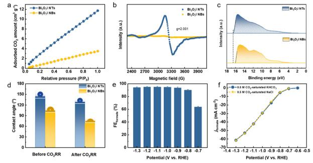
Fig. 6 (a)  $CO_2$  adsorption isotherms, (b) EPR spectra, (c) UPS spectra and (d) contact angle measurements before and after the  $CO_2RR$  on  $Bi_5O_7I$  NTs and NBs, (e) FE<sub>formate</sub> and (f)  $j_{formate}$  of Bi<sub>5</sub>O<sub>7</sub>I NTs in CO<sub>2</sub>-saturated 0.5 M NaCl.
