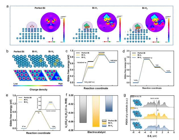
Fig. 5 DFT calculation results. (a) The electron density difference with \*OCHO adsorbates (2D view generated from the plane derived by Bi-O-O atoms), (b) electron local functions, Gibbs free energy of the CO<sub>2</sub>RR to (c) HCOOH pathway and (d) CO pathway, (e) Gibbs free energy of HER, (f) difference in limiting potentials for the CO<sub>2</sub>RR and HER, and (g) the Bi p-PDOS with \*OCHO adsorbates of perfect Bi, Bi-V<sub>1</sub> and Bi-V<sub>2</sub>.
