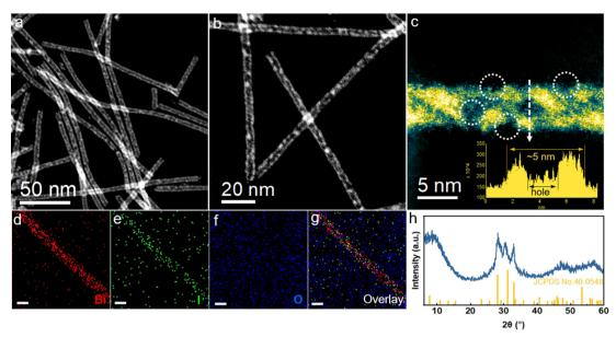
Fig. 1 Catalyst characterizations. (a-c) HADDF-STEM images of  $Bi_5O_7I$  NTs (inset is the line scan of the depth); (d-g) the corresponding EDS elemental mappings and overlay image of  $Bi_5O_7I$  NTs (scale bar: 5 nm); (h) XRD pattern of  $Bi_5O_7I$  NTs.
