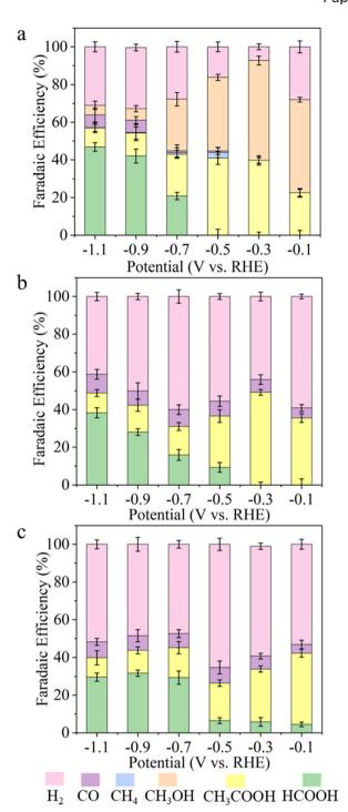
Fig. 6 Faradaic efficiency for all the liquid and gaseous products found during CO2 reduction as a function of potential on (a) AgBiS2 and (b) AgBiSe2 and (c) CuBiS2 catalysts in the flow cell configuration in 0.5 M KHCO<sub>3</sub>.
