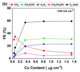
Fig. 3 Product distribution of the CORR as a function of the Cu loading in the electrodes at the current density of around 130 mA cm<sup>-2</sup> (a) and  $330 \text{ mA cm}^{-2} \text{ (b)}$
